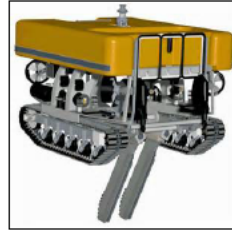
Figure 19 – ROV with Jetting Swords
