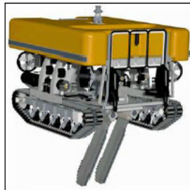
Figure 35 - ROV with Jetting Swords
