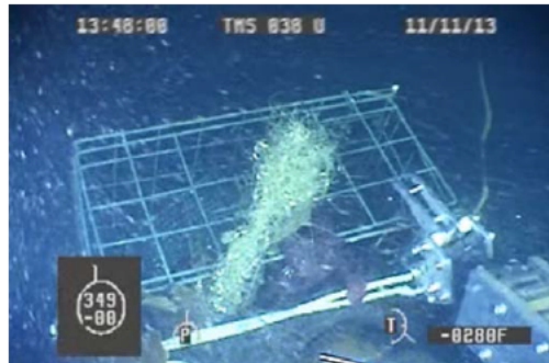
Figure 25 - Crab Pot Entangled with Cable
