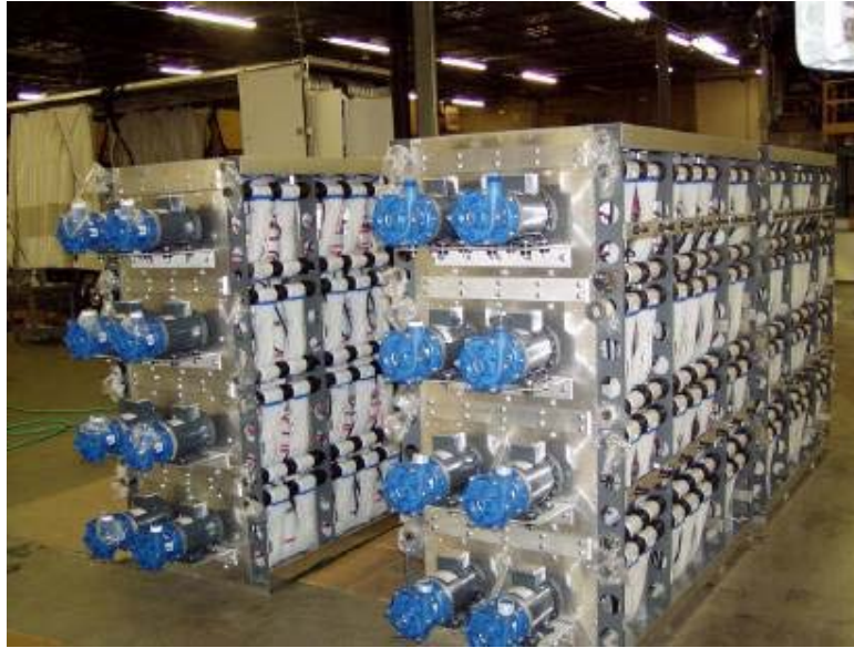
Figure 17- ZnBr Cell Stacks
