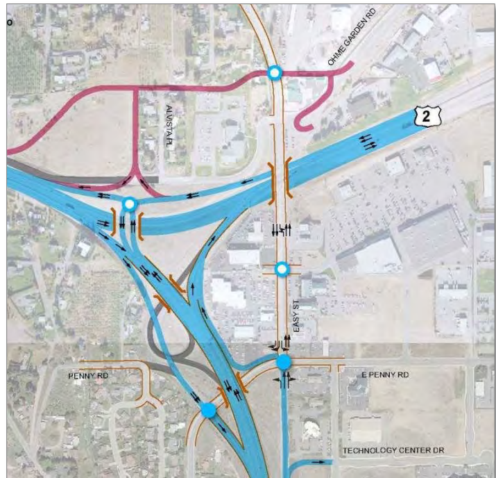
The North Wenatchee Transportation Master Plan recommends reconfiguring the US2 / SR 285 interchange to facilitate eastbound through traffic flows.
