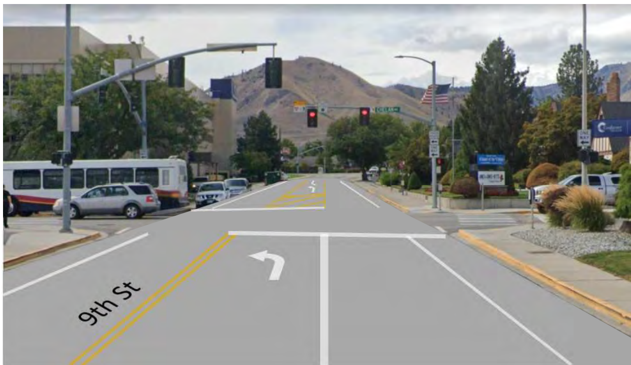
Figure 4-2. Conceptual view of 9th Street channelization near N Chelan Avenue (facing west).
