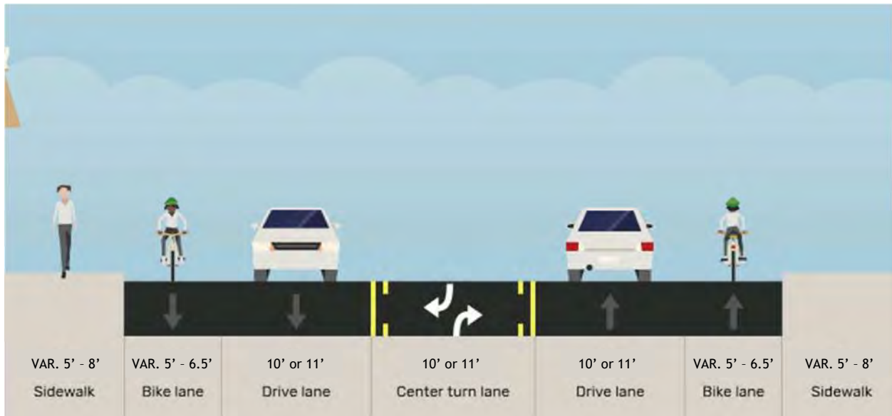
Figure 4-1. Preferred Alternative typical section.
