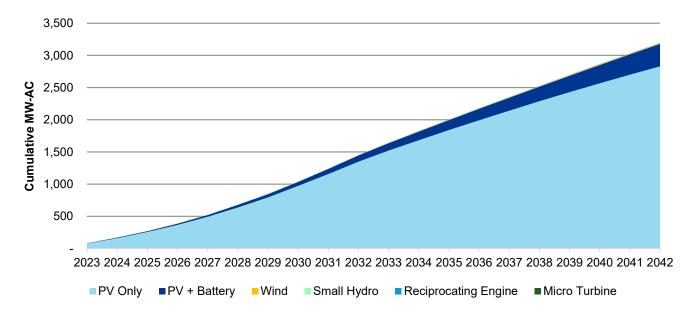
Figure 4-4 Cumulative New Capacity Installed by Technology (MW-AC), 2023-2042, High Case
