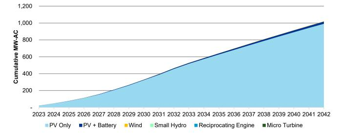
Figure 4-17 Cumulative New Capacity Installed by Technology (MW-AC), Oregon Base Case, 2023-2042
