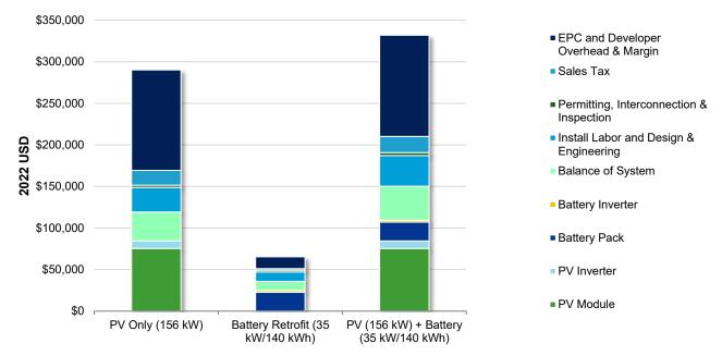
DNV has estimated all CapEx categories for the projects based on Wood Mackenzie's US 2022 H1 cost model, which has been found to be reasonable relative to actual CapEx that DNV has observed on projects it's reviewed in the past. DNV estimated the benchmark CapEx values based on the project capacity, location, and technology assumptions for each state and sector. When technology assumptions were unavailable, DNV made reasonable assumptions. Combined PV + Battery
