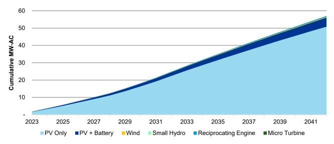
Figure 4-7 Cumulative New Capacity Installed by Technology (MW-AC), California Base Case, 2023-2042
