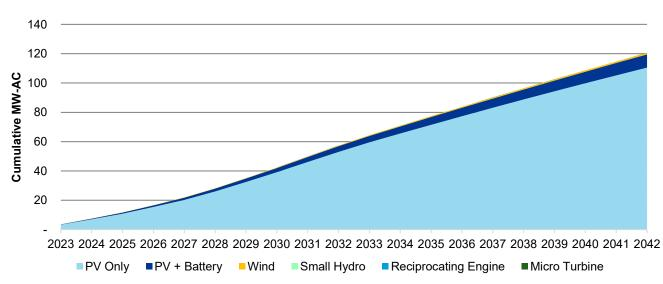
Figure 4-13 Cumulative New Capacity Installed by Technology (MW-AC), Idaho Low Case, 2023-2042
