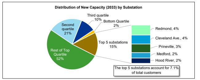
The top five of PacifiCorp's 193 substations account for 15% of 2033 forecast capacity (compared to 7% of customers), with the entire top quartile (representing 49% of customers) accounting for 67%.
