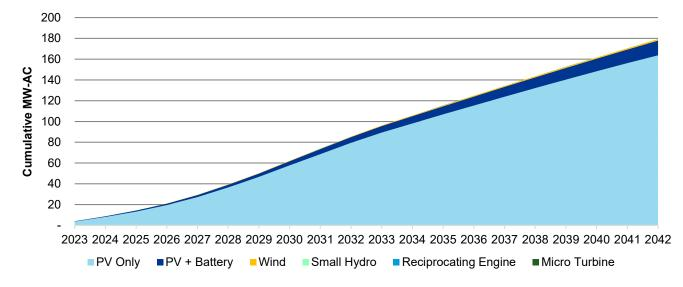
Figure 4-12 Cumulative New Capacity Installed by Technology (MW-AC), Idaho Base Case, 2023-2042
