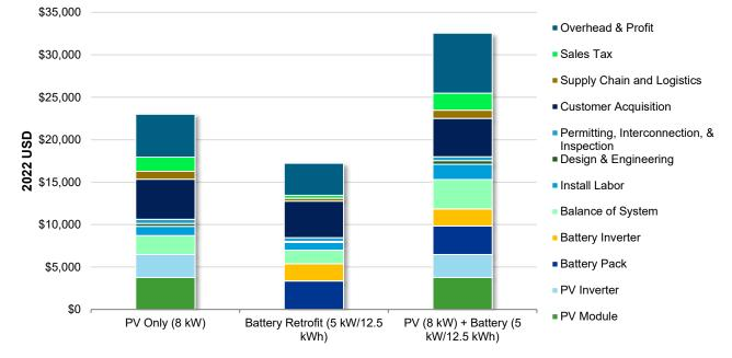
Figure 3-2 Cost of Residential PV Standalone, Battery Storage Retrofit to Existing PV, and PV + Battery Systems from DNV Bottom-up Cap-Ex Model, Utah
