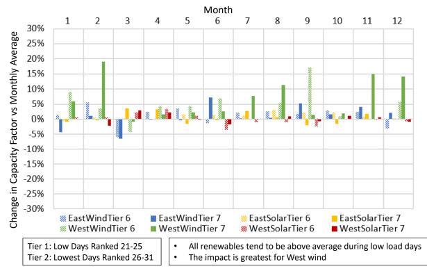
Standard stochastic evaluation of prices, loads, etc. is based on standard deviations and mean reversion statistics. The results indicate that wind and solar output does exhibit relationships with
