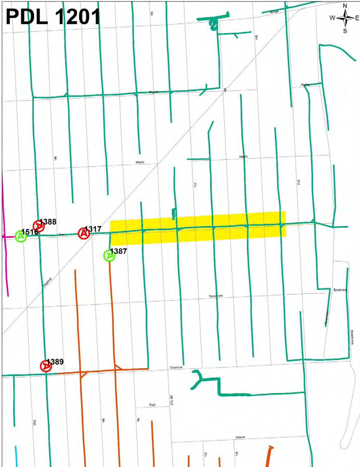
Figure 4. Polygon 5 Three-Phase Lateral Reconductor to 336 AAC
