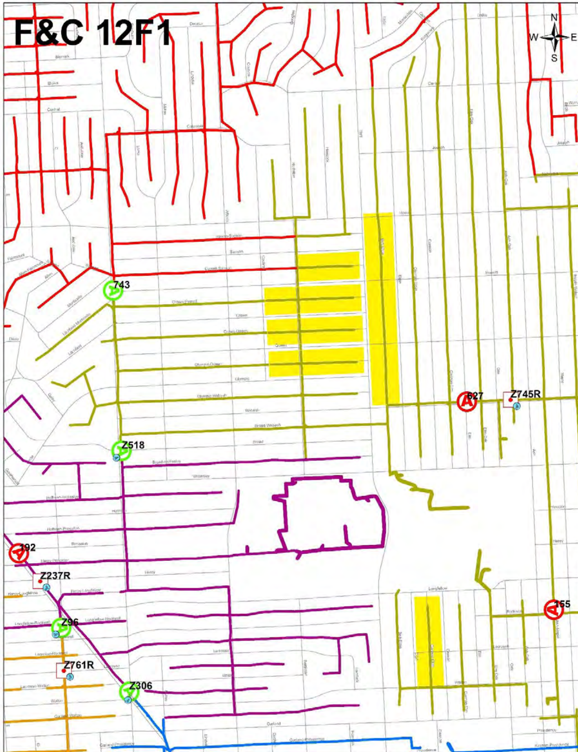
Figure 7. Laterals Requiring Field Analysis for Reconductoring to 4 ACSR
