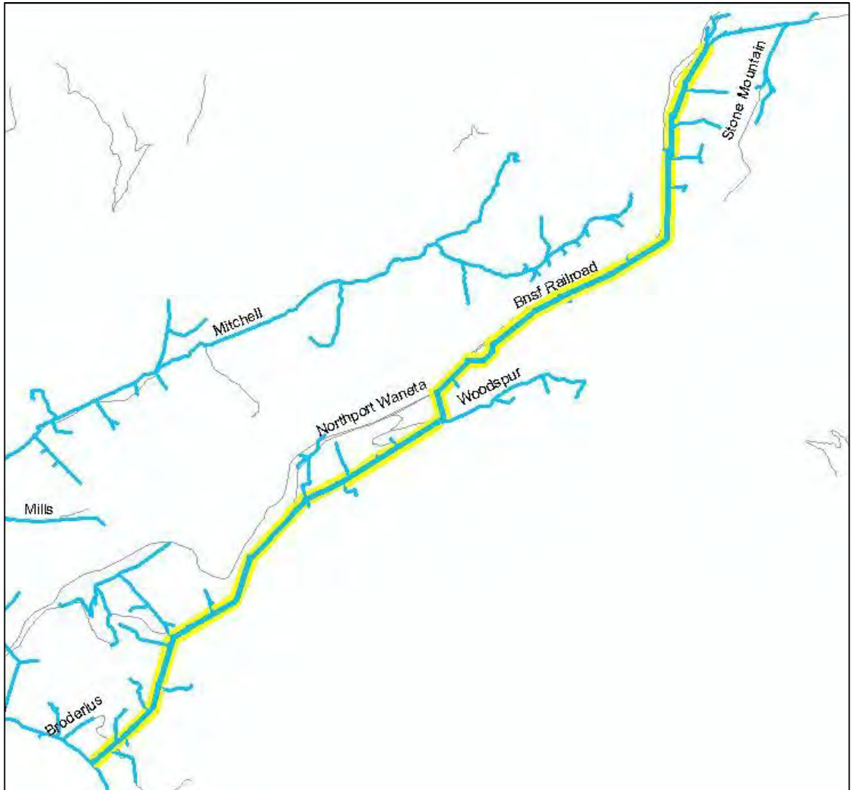
Figure 2. Section 1 Primary Reconductor to 4 ACSR
