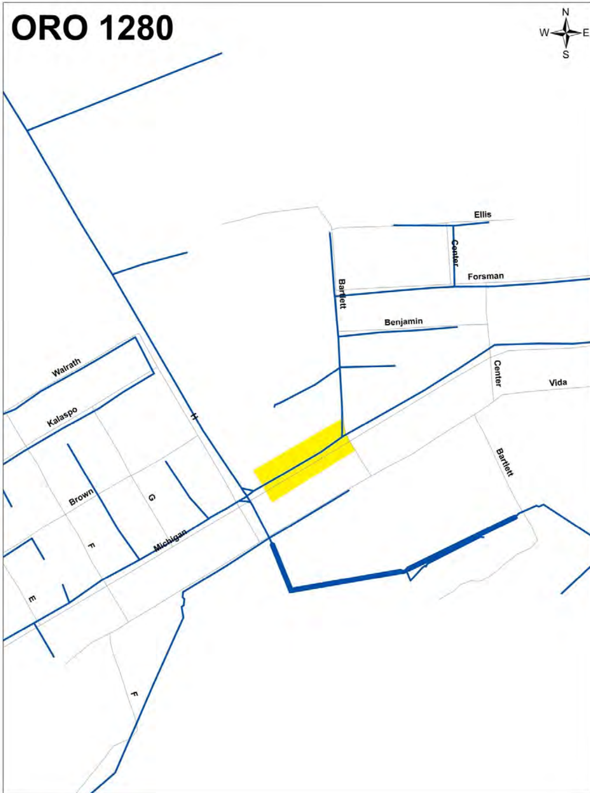
Figure 4. Polygon 5 Feeder Trunk Reconductor to 2/0 ACSR
