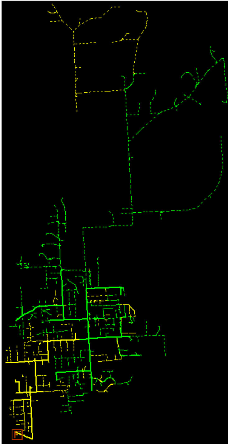
Figure 13. Modeled Voltage Levels at Peak Loading before Proposals
