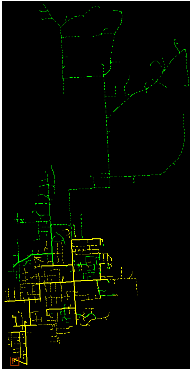
Figure 16. Modeled Voltage Levels at Average Loading after Proposals
