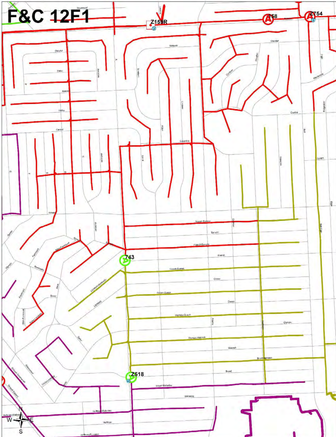
Figure 8. Feeder Tie Location near #743
