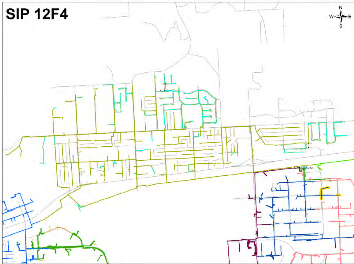
Figure 34. SIP 12F4 Identified Unknown URD Cable Segments
