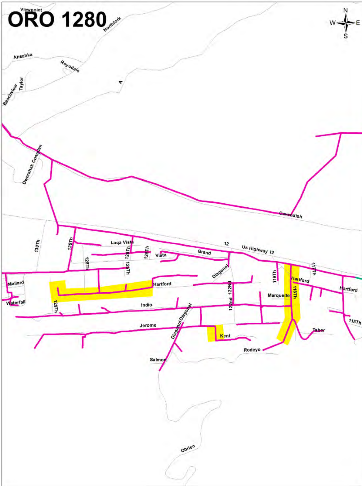
Figure 17. 6A Primary Laterals Requiring Reconductor
