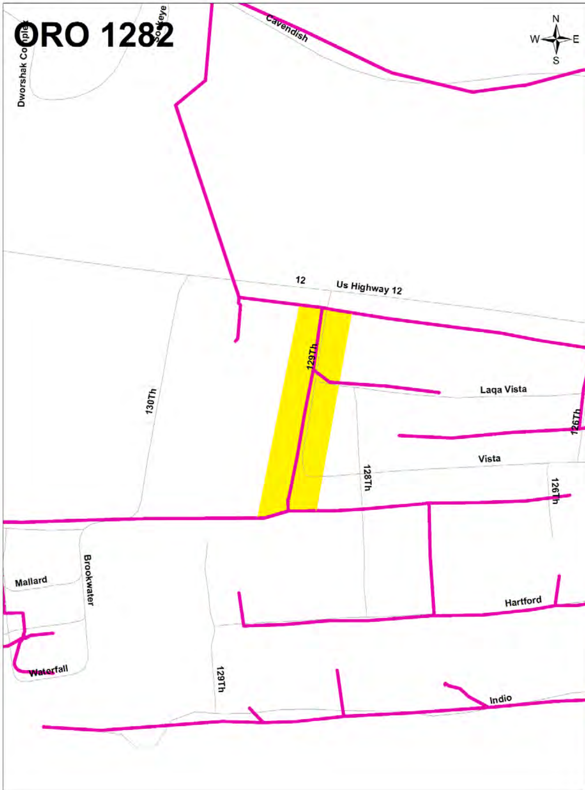
Figure 20. Install Additional Phase of 4ACSR Primary for Load Balancing
