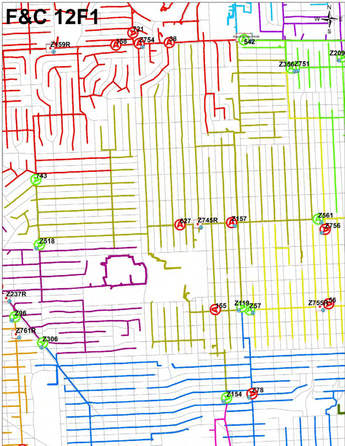
Figure 14. F&C 12F1 Automation Device Locations
