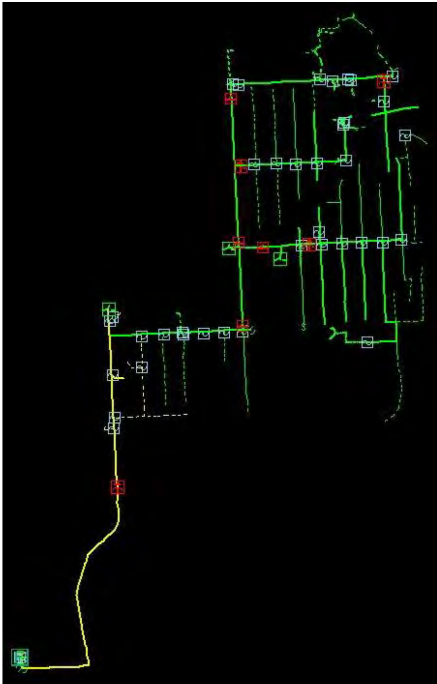
Figure 5. Modeled Voltage Levels at Peak Loading before Proposals
