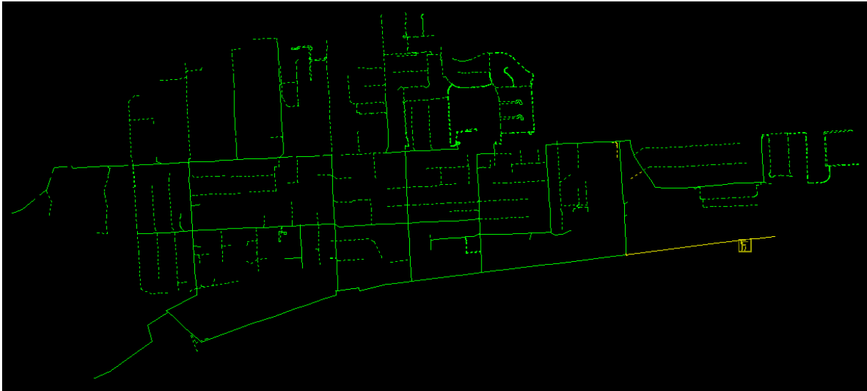
Figure 21. SIP 12F4 Modeled Voltage Levels at Peak Loading
