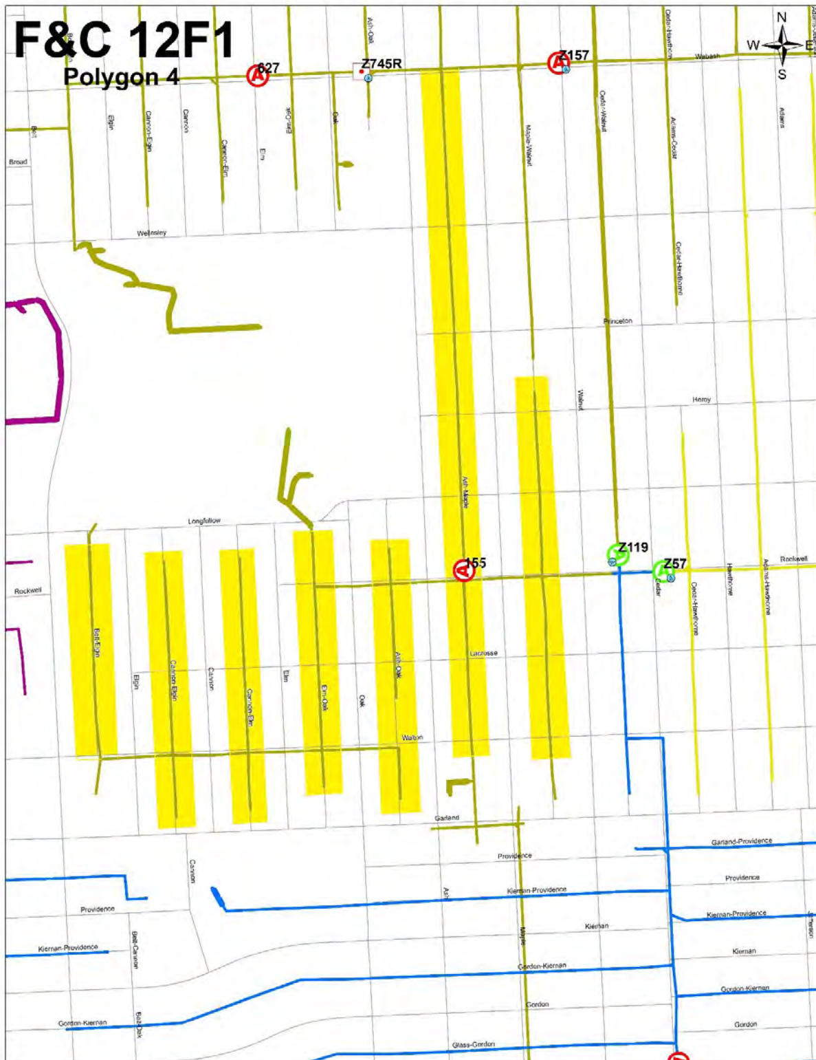
Figure 18. Open Wire Secondary Districts on Polygon 4 of F&C 12F1
