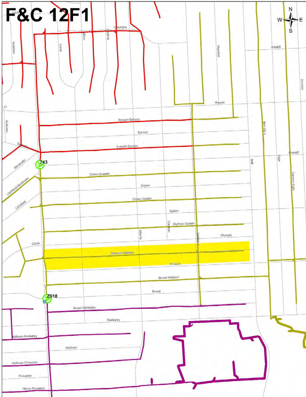
Figure 6. Polygon 5 Primary Lateral Recondutor to 4 ACSR
