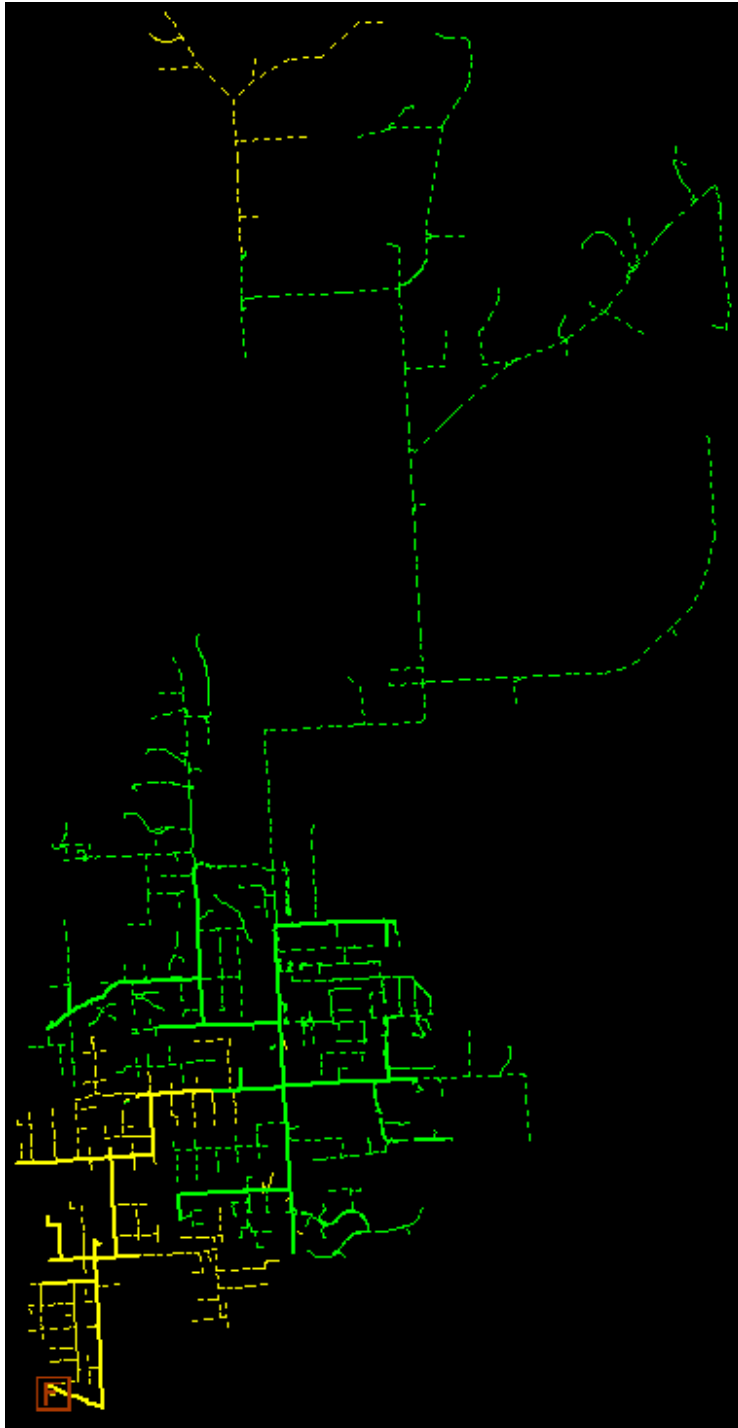
Figure 15. Modeled Voltage Levels at Peak Loading after Proposals
