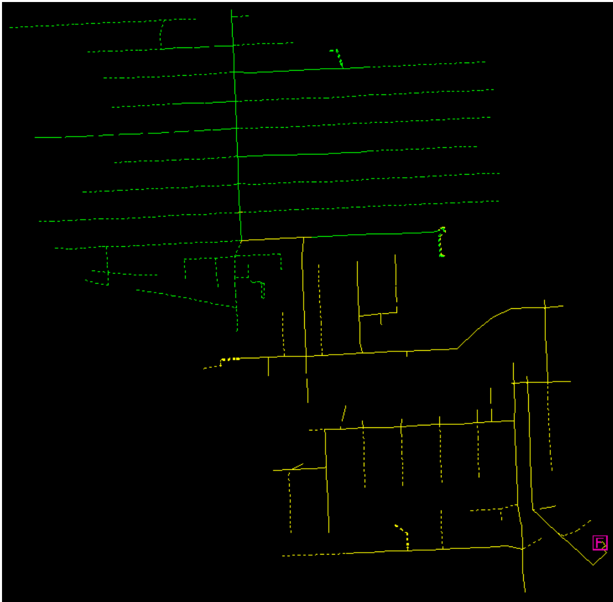
Figure 17. ROS 12F5 Modeled Voltage Levels at Peak Loading after Proposals
