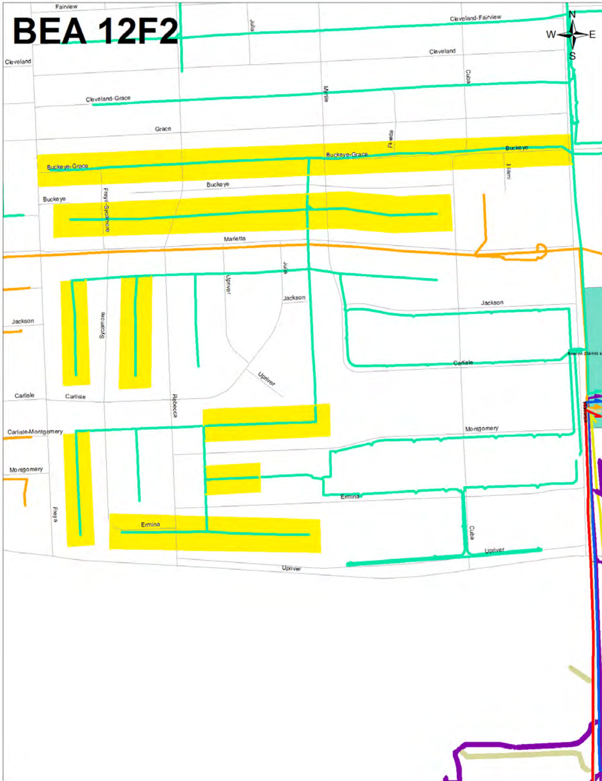
Figure 19. Open Wire Secondary Districts on Polygon 1 of BEA 12F2
