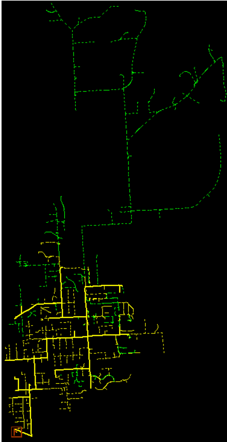
Figure 14. Modeled Voltage Levels at Average Loading before Proposals
