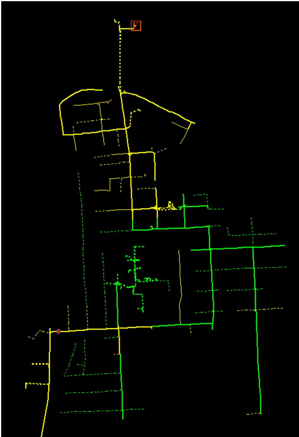
Figure 6. Modeled Voltage Levels at Peak Loading before Proposals – Serving SLW 1316 to the #1332 from HOL 1205
