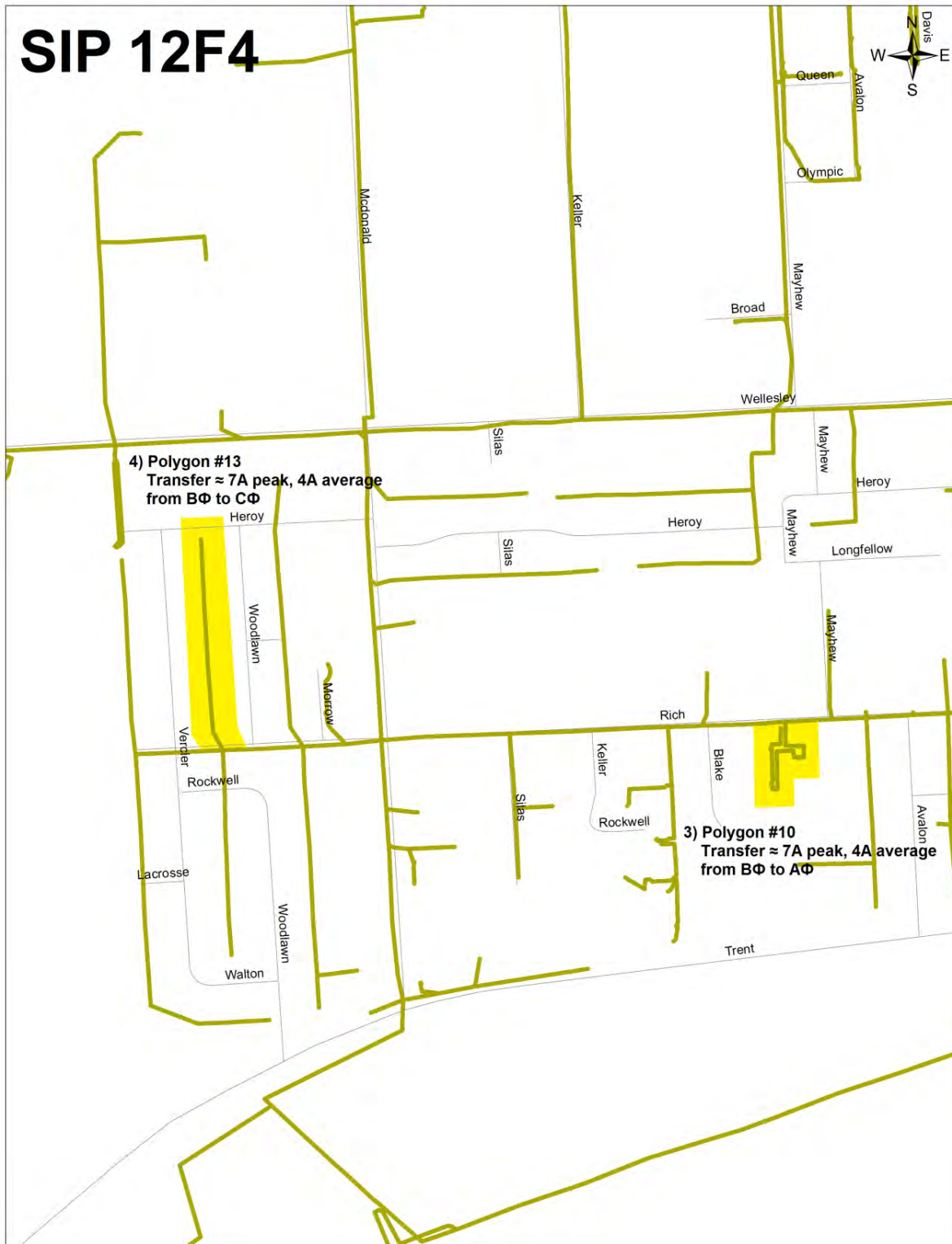
Figure 11. SIP 12F4 Load Balancing on Polygons 10 and 13
