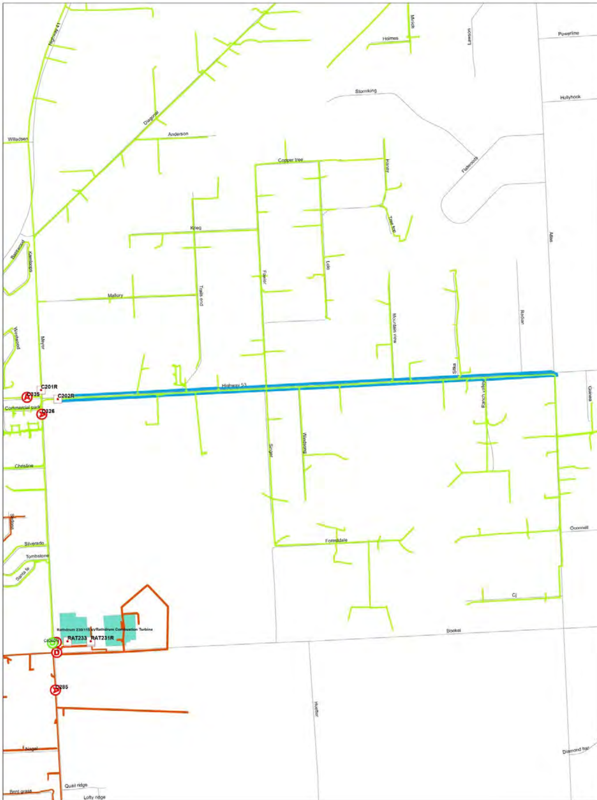
Figure 3. Polygons 2 and 4 Primary Reconductor to 2/0 ACSR
