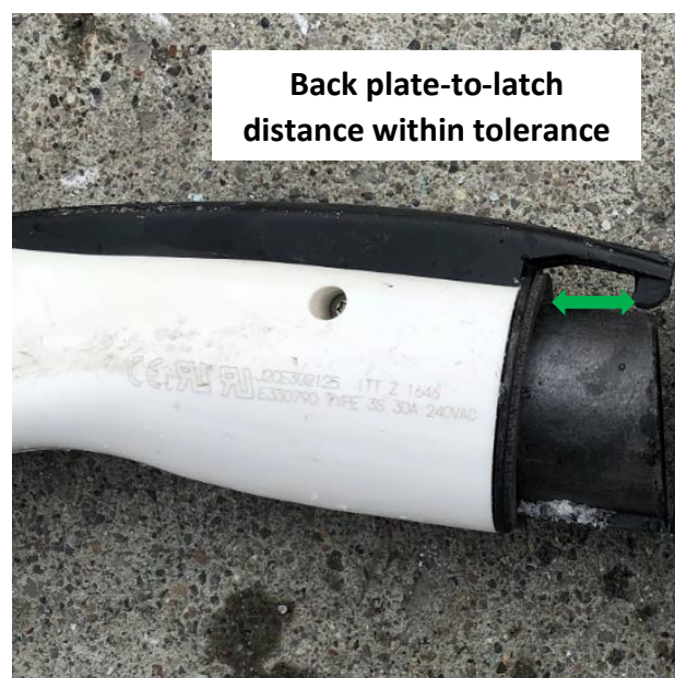
Figure 30. Example J1772 connector plate-to-latch tolerance
