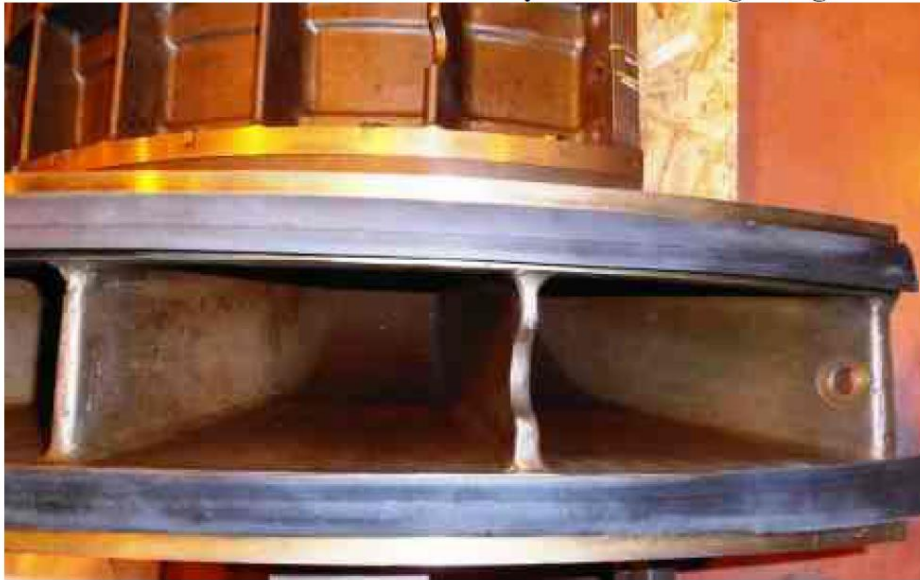
5 RS Generator Blower Stationary Blade Casting Gouges
