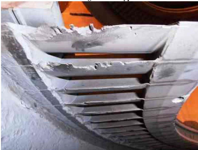
15 Governor UH Blade Ring 1 Row 1 Typical FOD to Blades
