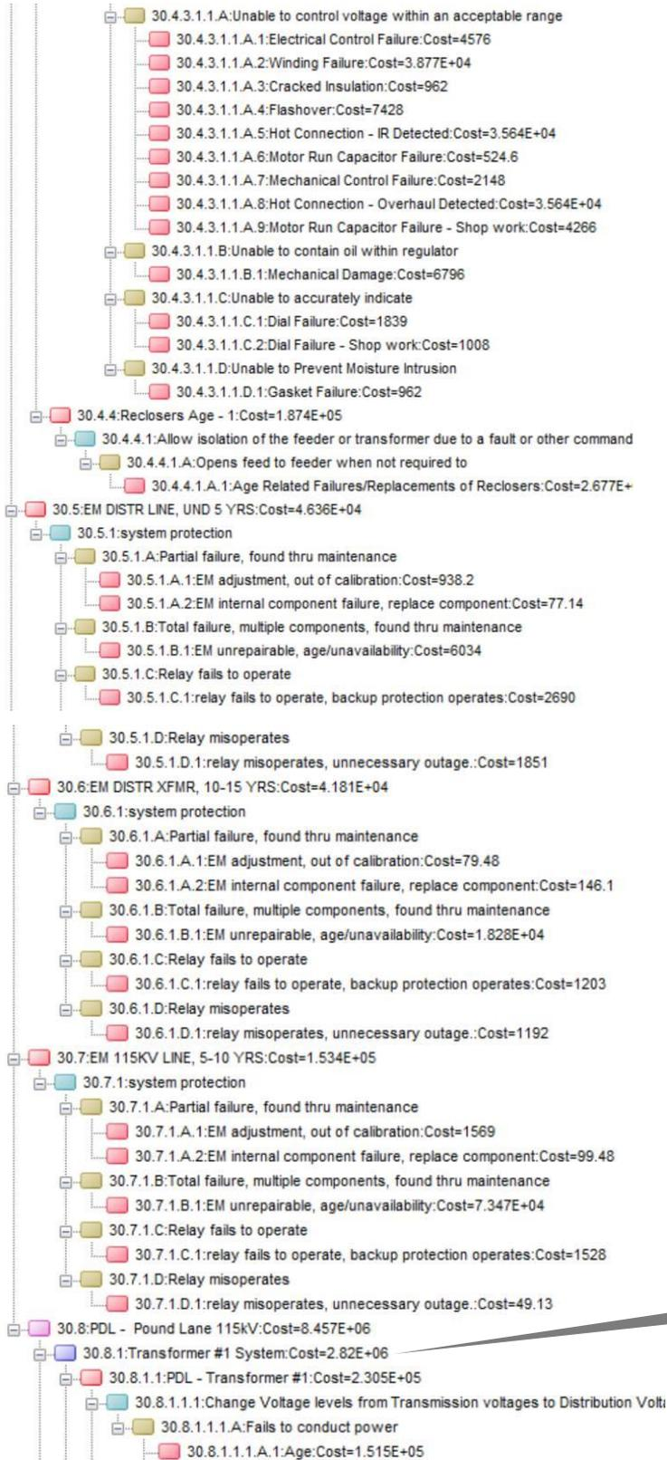
Pound Lane Substation Transformers #1 and #2 are shown in this portion of the directory. The Availability Workbench model directory is similar in appearance to that shown above for regulators, however, the transformers include different purpose statements and have unique characteristics for the equipment type ages, failure modes and costs.
