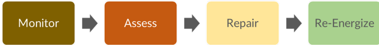
Figure 18: General Re-Energization Process
