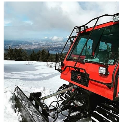
Snowcat plows a path for line crews
