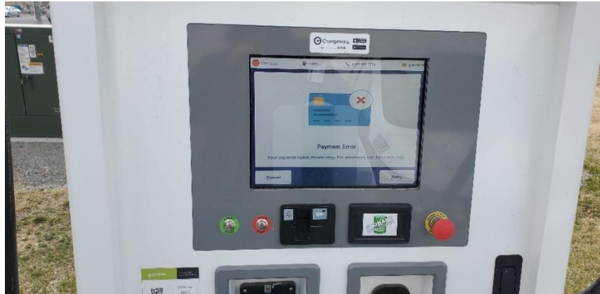
Figure 18: DCFC station with payment error displayed on user interface (U/I) screen
