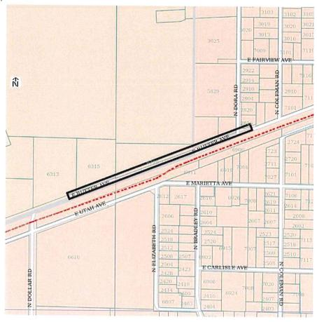
M&L Construction was performing directional bore work in front of the "lifeflight" headquarters at Felts Field. We decided to spend the effort to stay as far away from the gas line as possible due to the lack of trust in Avista's locate capabilities and the critical businesses located here.
