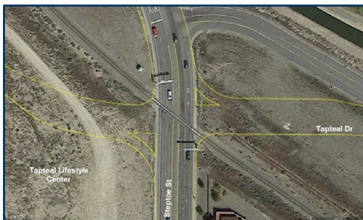
Figure 5 - Alternative 2: Four-Leg Intersection
