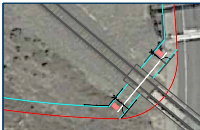
Figure 11 - Example pedestrian emergency exit gates
