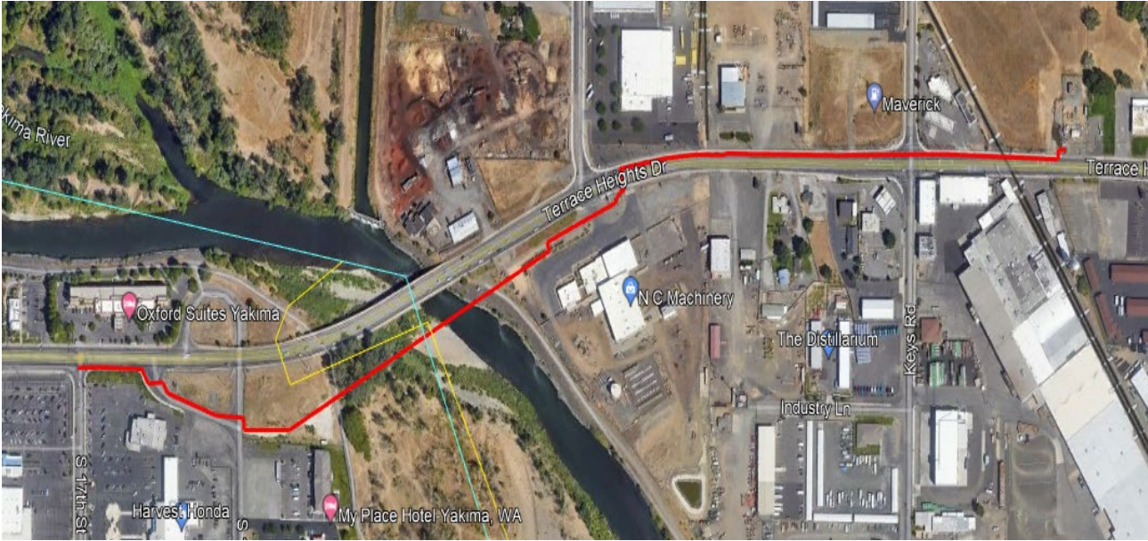
Figure 1: Overall view of the proposed 8” Yakima HP Replacement (Red) pipeline alignment.
