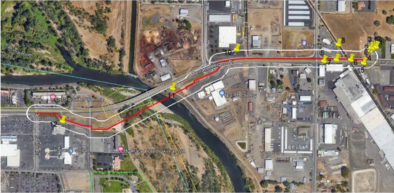
Figure 2: Section of the proposed pipeline showing buildings 1-12 within the 100-foot proximity boundary.
