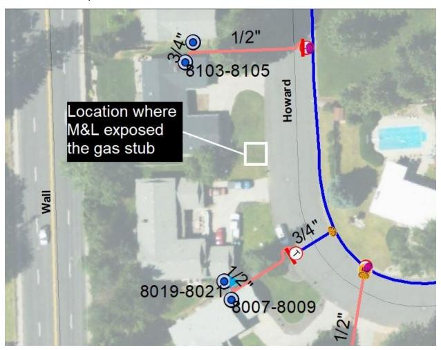
Avista locate request to determine accurate location of stub:
