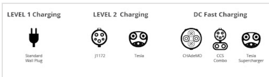
Figure 8: Power Levels and Connector Standards for EV Charging in North America
