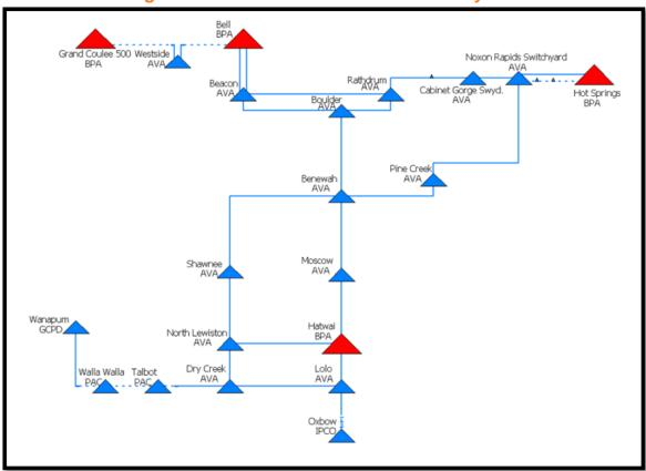
Figure 7.2: Avista 230 kV Transmission System
