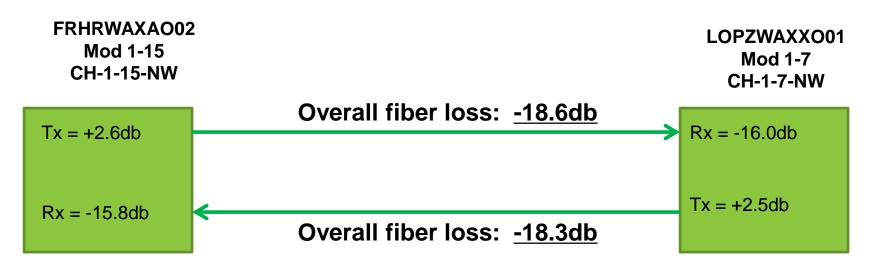
SFP Specifications SFP/2G5U/C1570V/SM/LC Transmitter output power range 0 dBm ... +4 dBm Receiver dynamic range -22 dBm ... -9 dBm SFP Specifications SFP/2G5U/C1490V/SM/LC Transmitter output power range 0 dBm ... +4 dBm Receiver dynamic range -22 dBm ... -9 dBm
