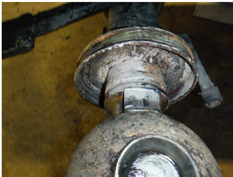
Stretch Duck axle with 2003 Ride the Ducks International modification
