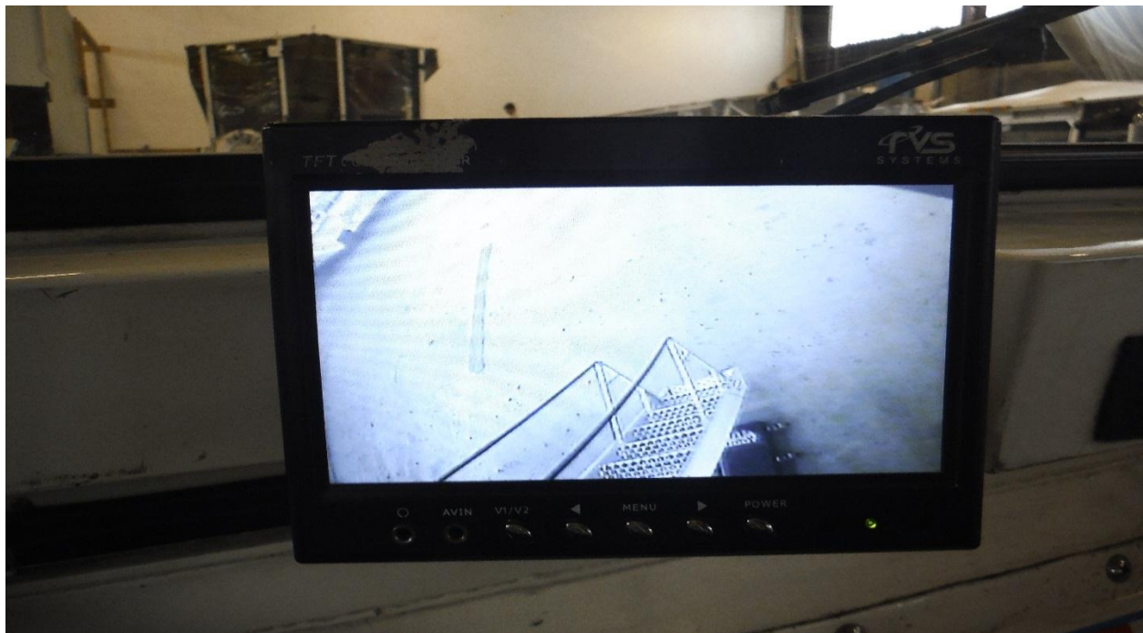
Duck Vehicle driver video screen – rear camera view
