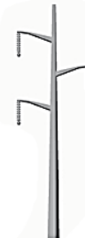
Transmission Nominal Voltage: 345 kV Type: Double Ckt Pole Typical Tower Height: 115-150 feet Typical Right-of-Way Width: 140-160 feet
