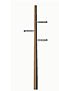
Transmission Nominal Voltage: 115 kV Type: Single Pole Typical Tower Height: 55-80 feet Typical Right-of-Way Width: 90-130 feet
