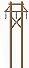
Transmission Nominal Voltage: 230 kV Type: H-Frame Typical Tower Height: 60-90 feet Typical Right-of-Way Width: 100-160 feet
