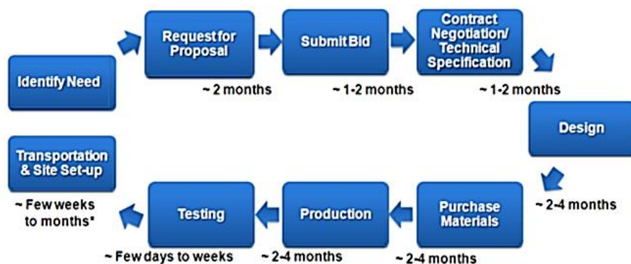
Large Power Transformer Procurement Process and Estimated Lead Time – Not Including Installation Time
