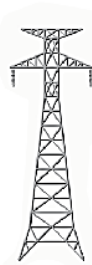
Transmission Nominal Voltage: +/- 400 kV HVDC Type: Tower Typical Tower Height: 145-180 feet Typical Right-of-Way Width: 160-180 feet
