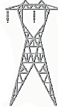
Transmission Nominal Voltage: 500 kV Type: Tower Typical Tower Height: 90-150 feet Typical Right-of-Way Width: 160-200 feet
