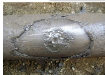
Steel Pipe Corrosion Damage
