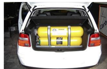
Compressed Natural Gas Tank
