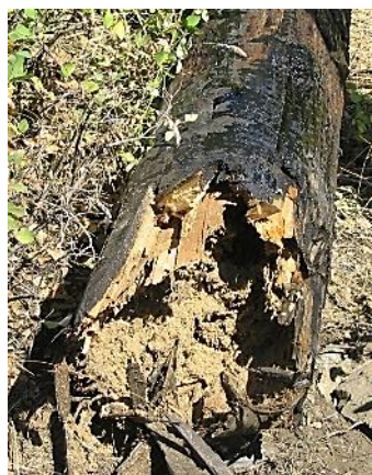
Above: A pole rots and fails Below: Replacing old pole with new (significantly straighter) pole Top Right: Pole hit by a truck Bottom Right: Wind storm causes a pole to split
