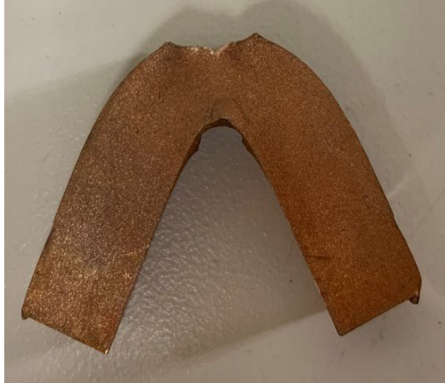
Figure 109: Photo of Charpy Tested Cu Alloy
