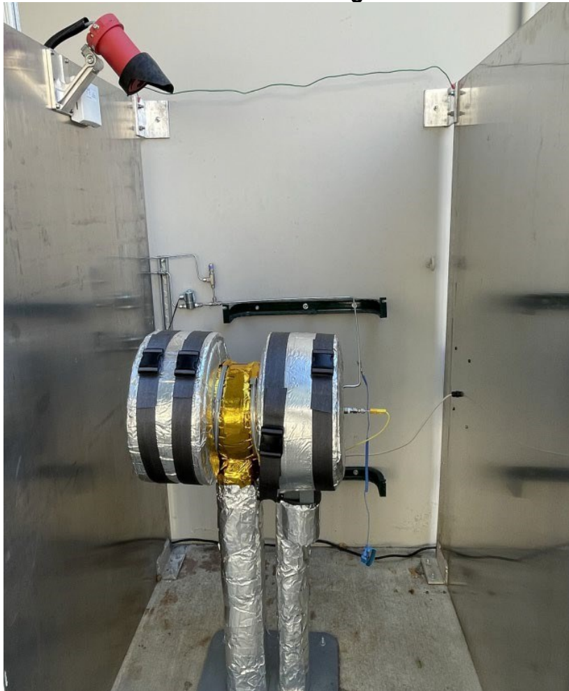
Figure 83: View of Test Chamber with Heating Element and Thermal Insulation
