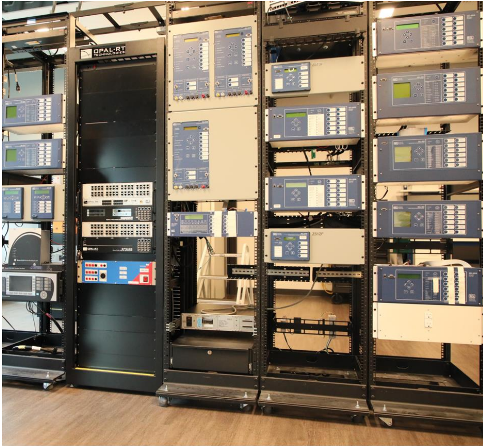
Figure 3 - Real-time simulation environment in the Avista Energy Innovation Lab
