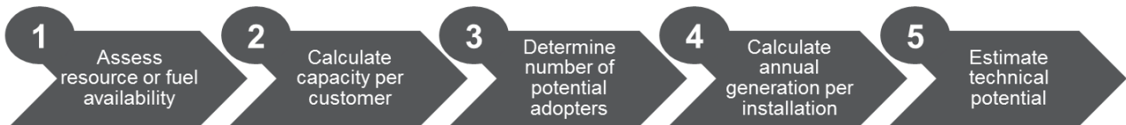
Figure 11. Technical Potential Approach
