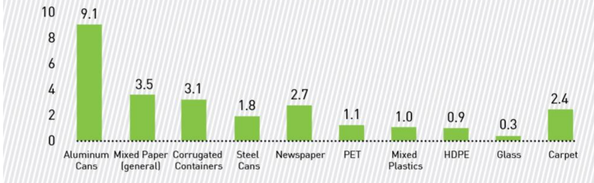
Figure 4.5: Same weight, different impacts. Using data on tons recycled to calculate environmental impacts can help a community make better-informed choices about what to include on their accepted materials list. The graph shows equivalent metric tons of CO 2 reduced for each ton recycled. Taken from the 2018 Waste Management Sustainability Report . Data calculated using EPA's WARM model .
