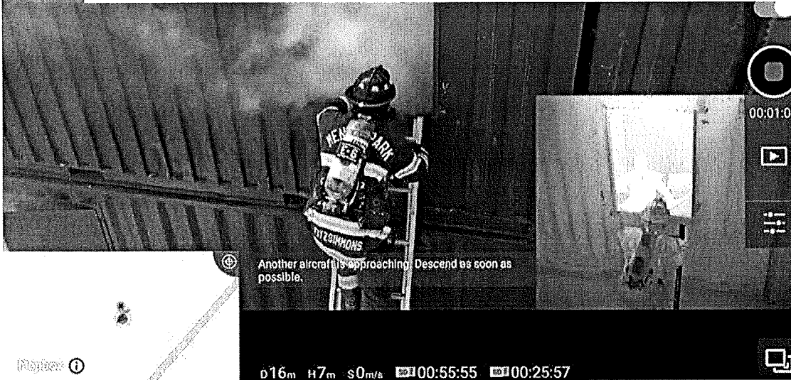
6 The Zenmuse XT2 camera carried by a DJI drone can show both regular view and infrared images at the same time. (Photos 6 and 7 courtesy of DJI.)
