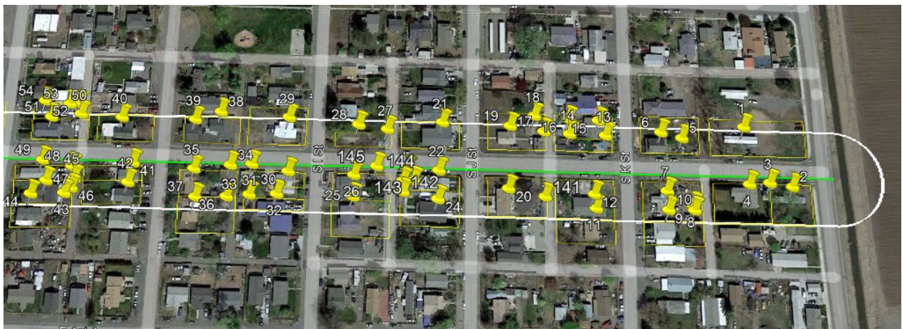
Figure 2: Section of the proposed pipeline from N. Meyers Rd to S. G St showing buildings within the 100-foot proximity boundary.
