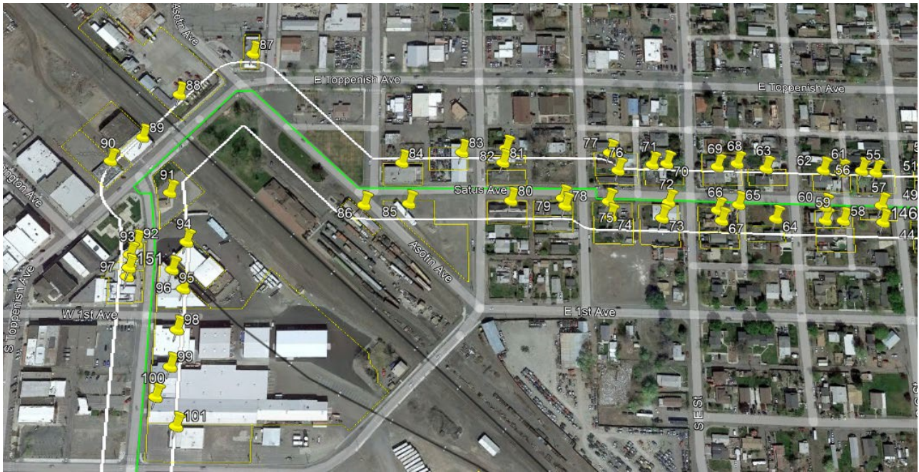
Figure 3: Section of the proposed pipeline from S. G St to W. 2 nd Ave showing buildings within the 100-foot proximity boundary.
