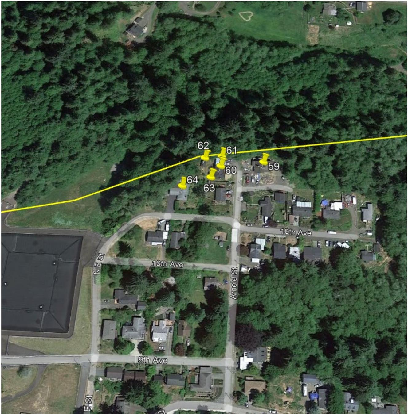
Figure 4: Section of the proposed pipeline showing buildings 59-64 within the 100-foot proximity boundary.
