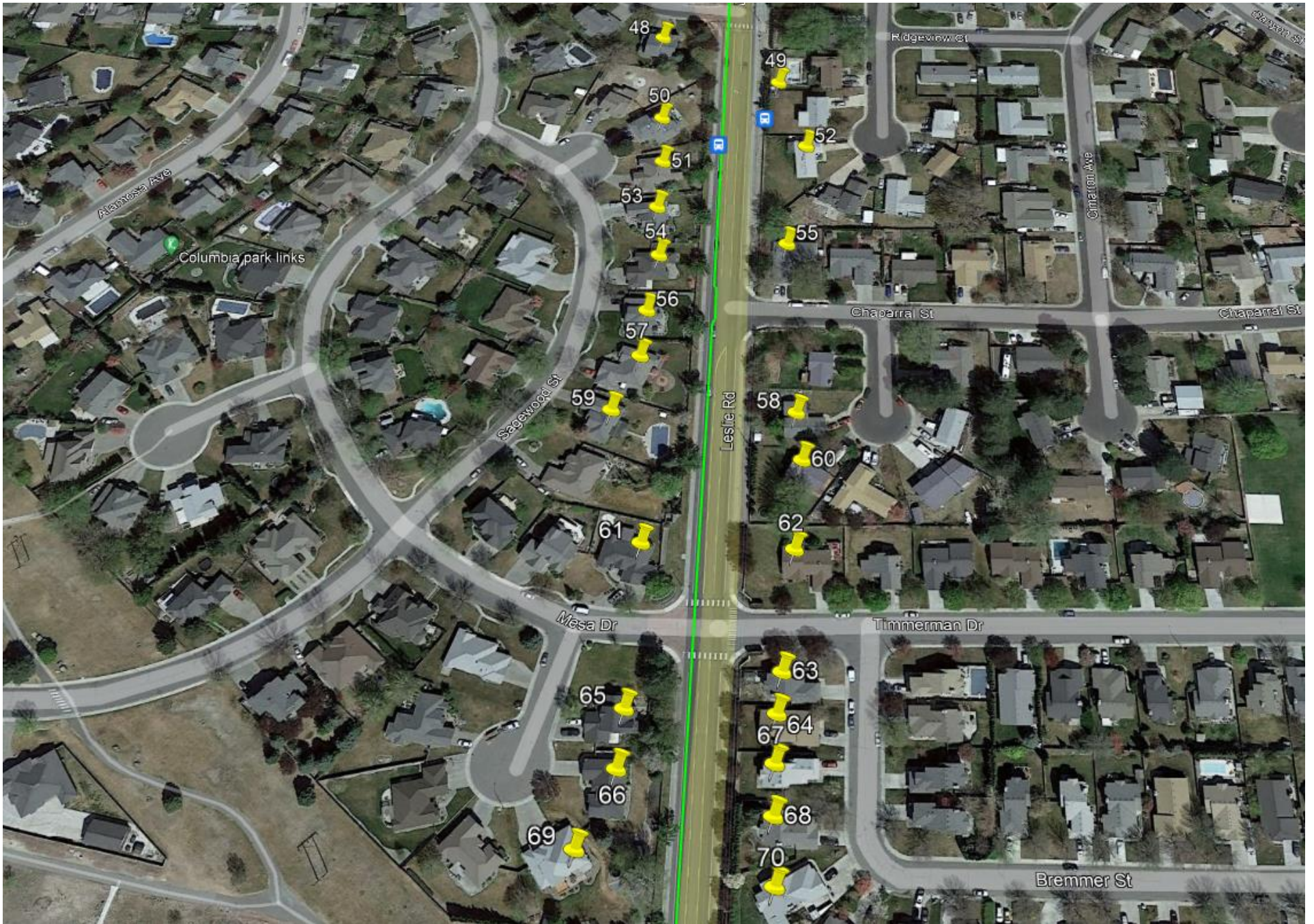
Figure 6: Section of the proposed Richland HP Lateral showing its proximity to buildings 48-70 within the 100-foot boundary.
