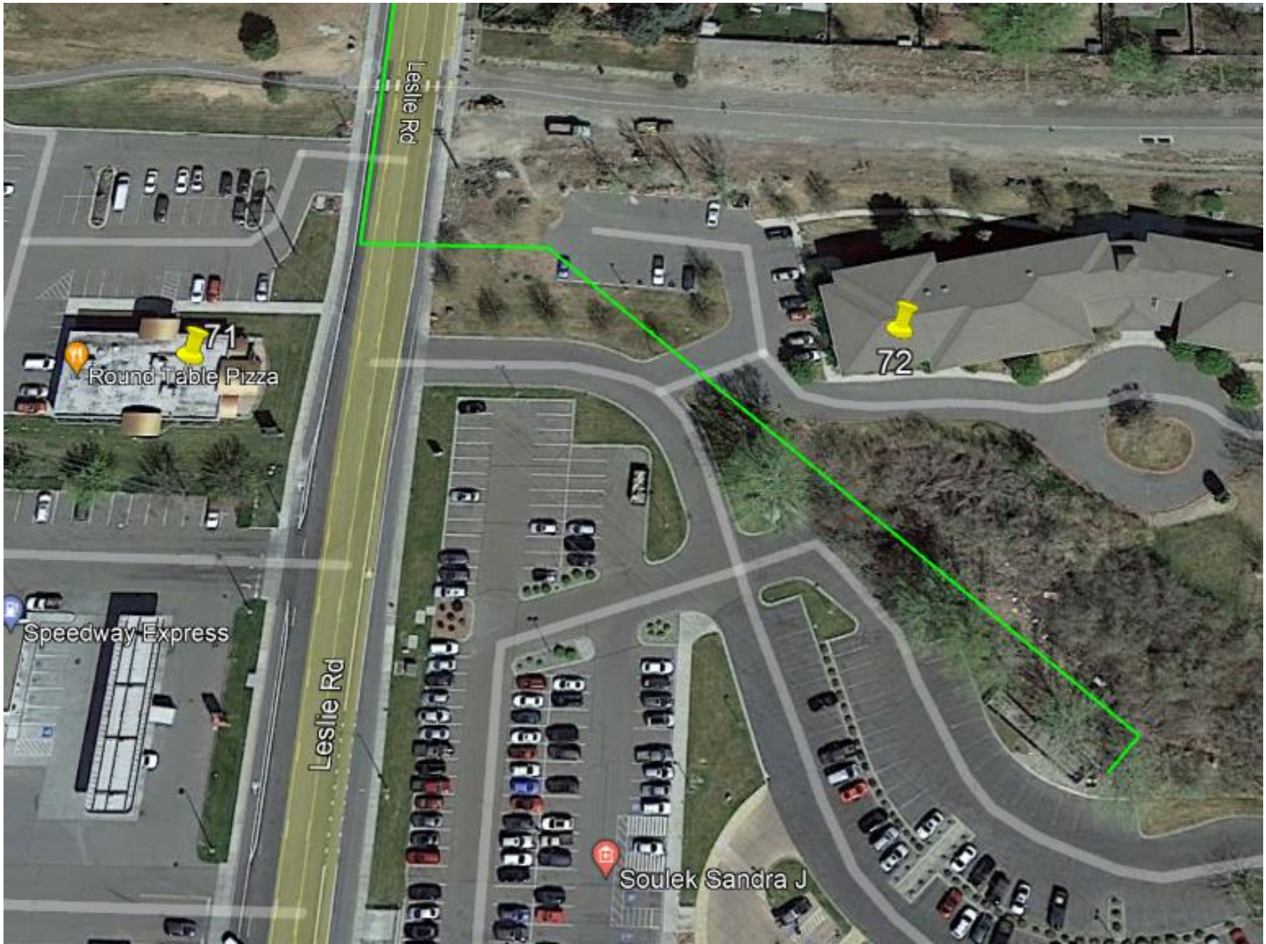
Figure 7: Section of the proposed Richland HP Lateral showing its proximity to buildings 71 and 72 within the 100-foot boundary.
