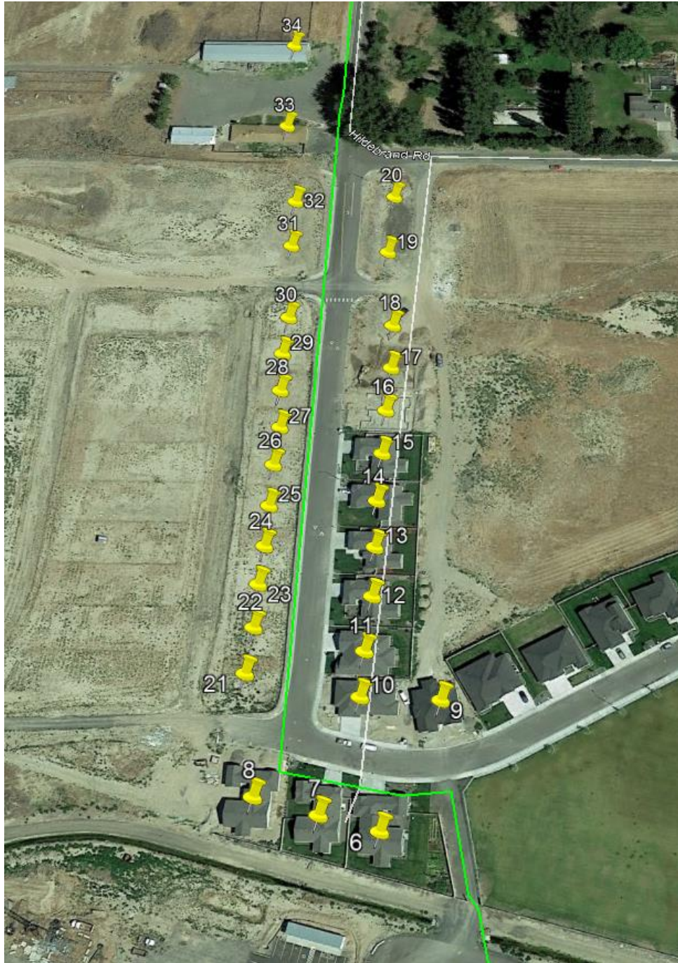
Figure 3: Second section of Southridge HP showing buildings 6-34 within the 100-foot proximity to the pipeline.
