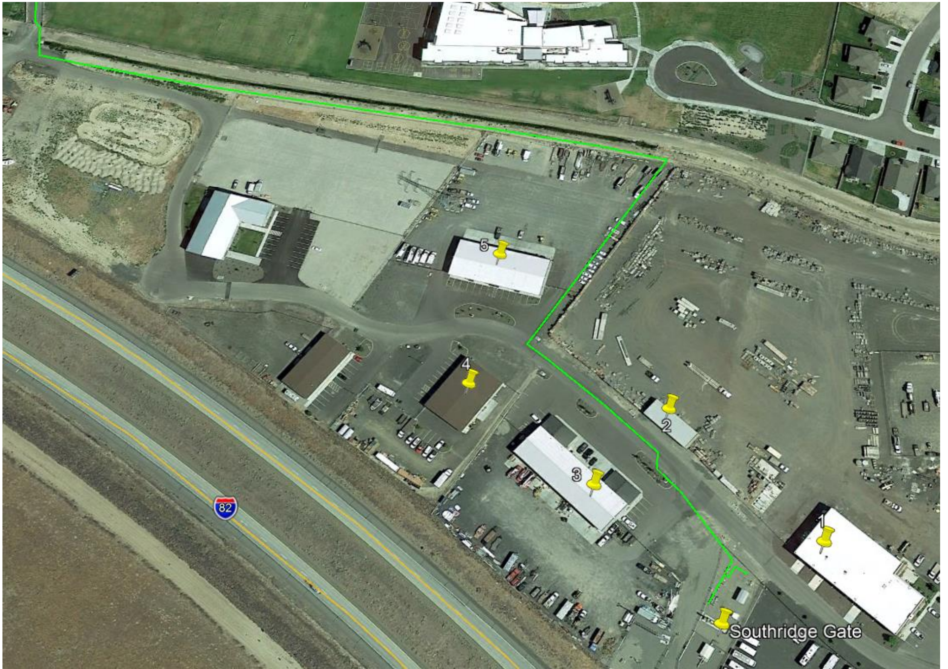
Figure 2: First section of Southridge HP line feeding from the Southridge gate station containing buildings 1-5 within the 100-foot proximity to the pipeline.
