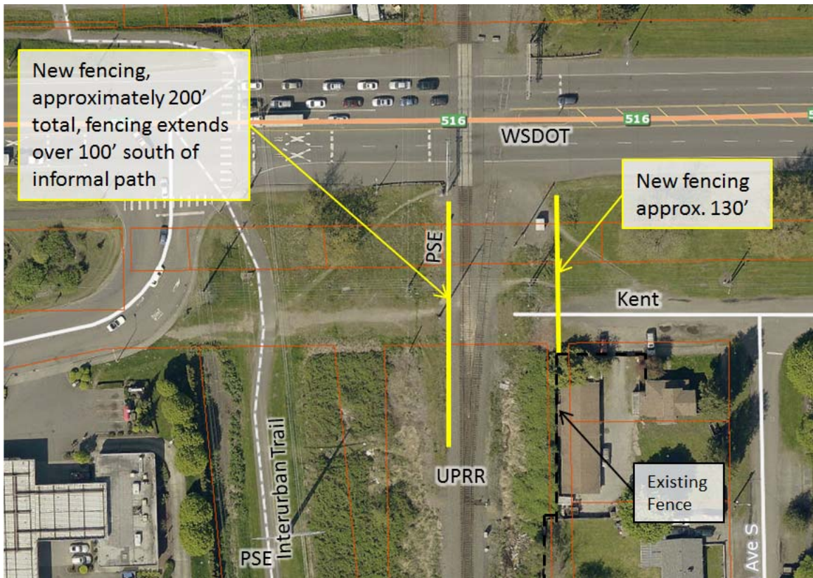
New fencing will help to eliminate unauthorized crossings.
