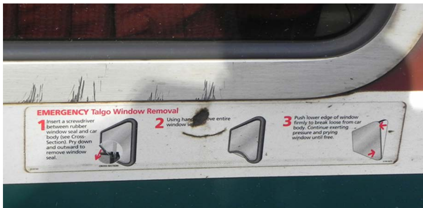
Figure 39. Interior emergency window removal instructions.
