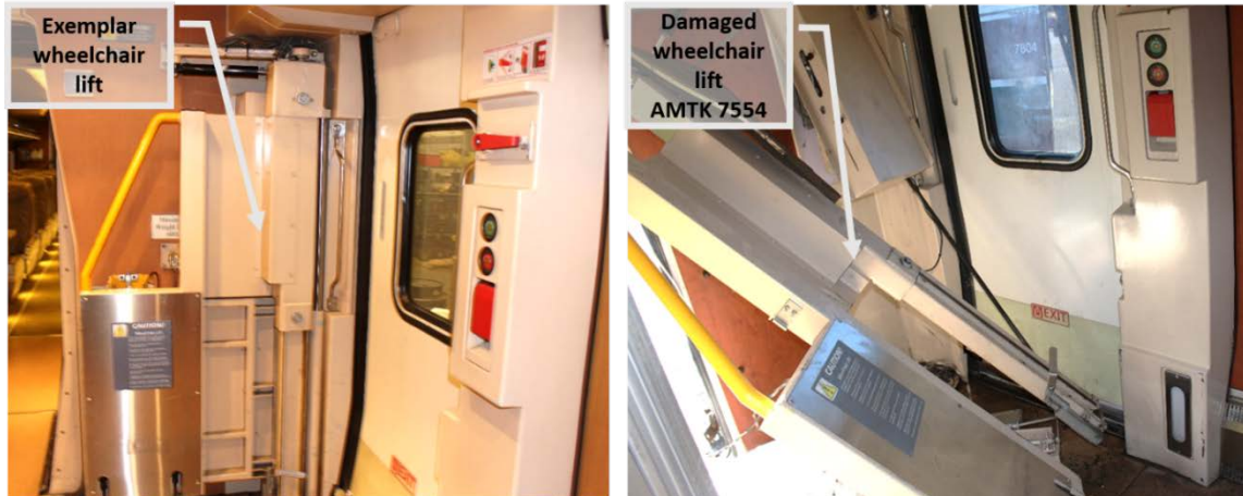
Figure 33. Exemplar wheelchair lift and damaged lift in AMTK 7554 (4).
