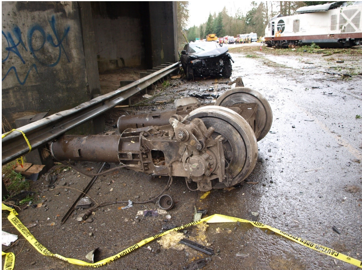
Figure 25. Detached rolling assembly and Grand Cherokee. (Photo provided by WSP.)
