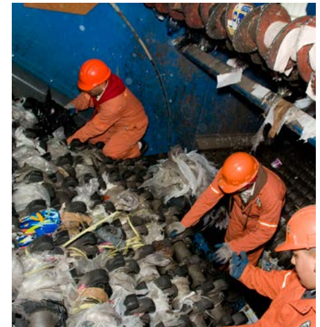
The sorting equipment is filled with plastic bags. Twice a day employees have to shut down the entire system so they can crawl onto the screen and use knives to cut away the plastic (Waste Connections)
