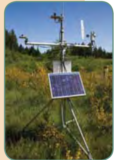
Powered by solar panels, weather stations provide data to support environmental monitoring and maintenance at several division facilities.
