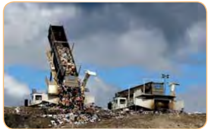
Side-by-side tippers greatly reduce the time required for unloading garbage trailers at the landfill.
