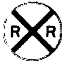
Figure 8B-2. Advance Warning Signs
