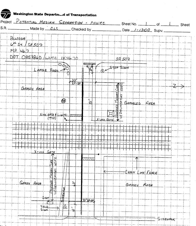
Prefabricated rubber/plast. curb units anchored to pavement. Notes: N. MAIN ST. Curb is 12" wide # 3 1/2 to 4" high with Delinators (Reboundable) a mountable cross Section. Curbs have 135 to 4" (mountack) reflectors attached to Elevation their top. Yellow is the CURB Details Vary
