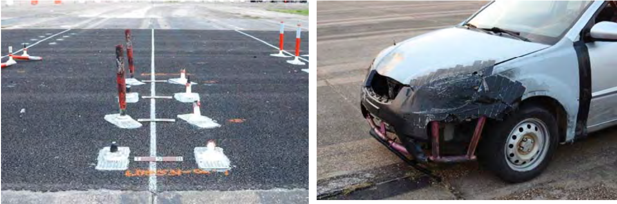
Figure 3.38. 607531-02-9 Delineators and Test Vehicle after Testing (Asphalt Surface).
