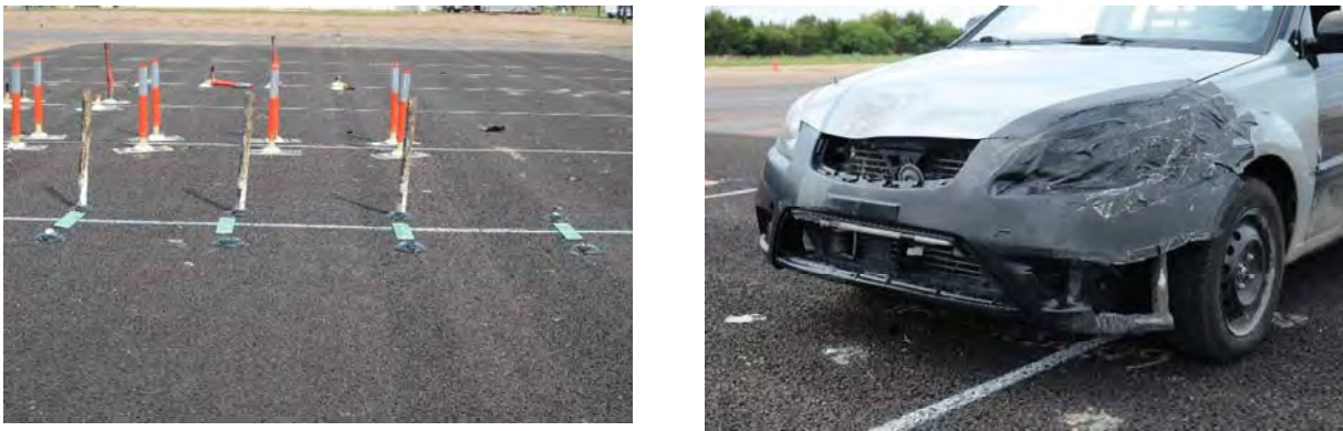
Figure 3.41. 607531-02-10 Delineators and Test Vehicle after Testing.
