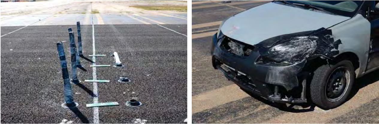
Figure 3.49. 607531-02-11 Delineators and Test Vehicle after Testing (Asphalt Surface).
