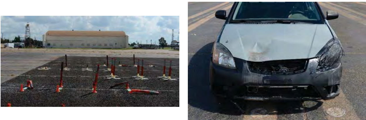
Figure 3.9. 607531-2 Delineators and Test Vehicle after Testing.
