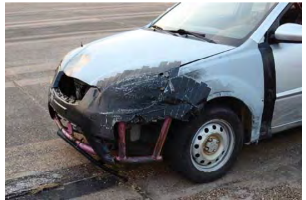
Figure 3.36. 607531-02-9 Delineators and Test Vehicle after Testing (Concrete Surface).
