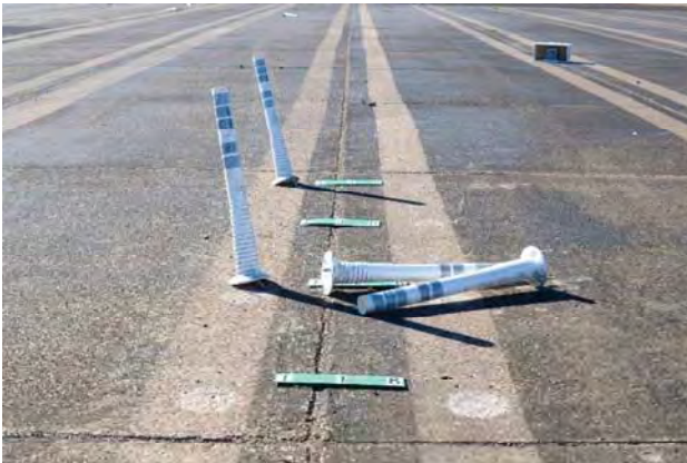
Figure 3.47. 607531-02-11 Delineators and Test Vehicle after Testing (Concrete Surface).
