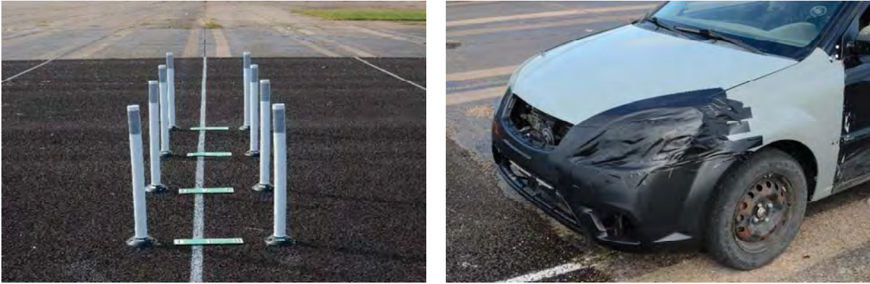
Figure 3.40. 607531-02-10 Delineators and Test Vehicle before Testing.
