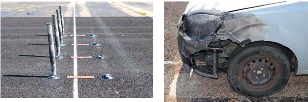
Figure 3.24. 607531-02-5 Delineators and Test Vehicle after Testing.
