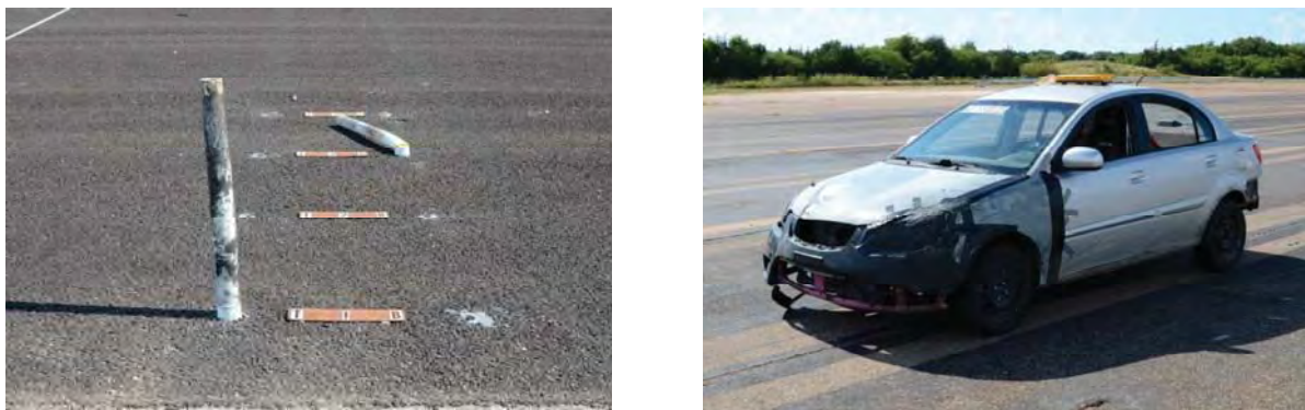
Figure 3.13. 607531-02-3 Delineators and Test Vehicle after Testing.
