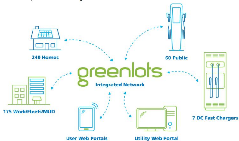
Figure 6: Integrated EVSE network design for the EVSE pilot (2016—2019)
