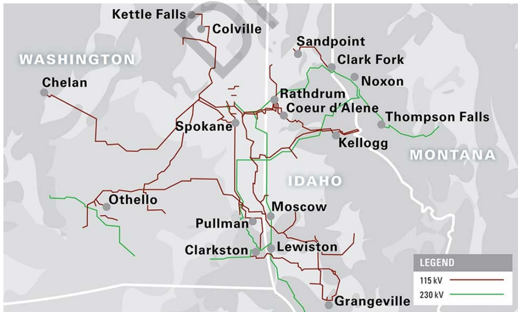
Figure 7.1: Avista Transmission System
