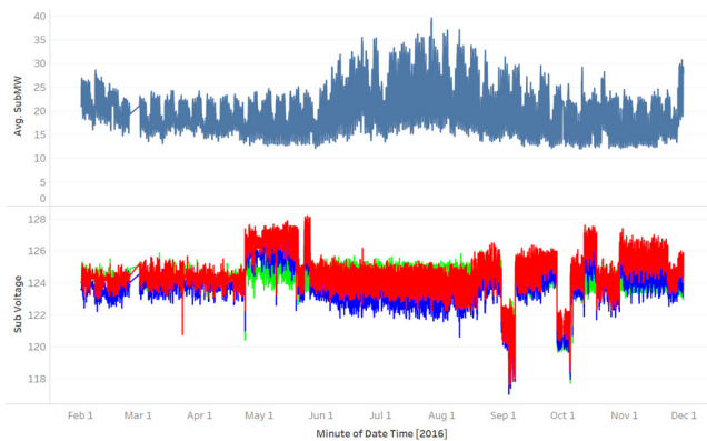
Fig. 2. Yearly substation MW and voltages by phase
