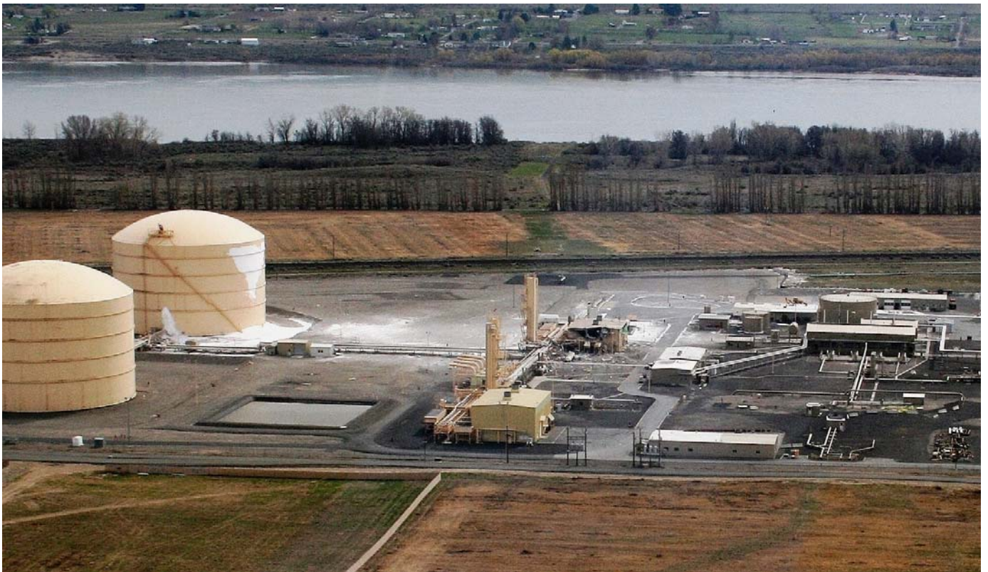
Aerial view taken shortly after the failure. Fires still burning. Perlite insulation leakage from the penetrated outer LNG-1 storage tank. Control room lower left.
