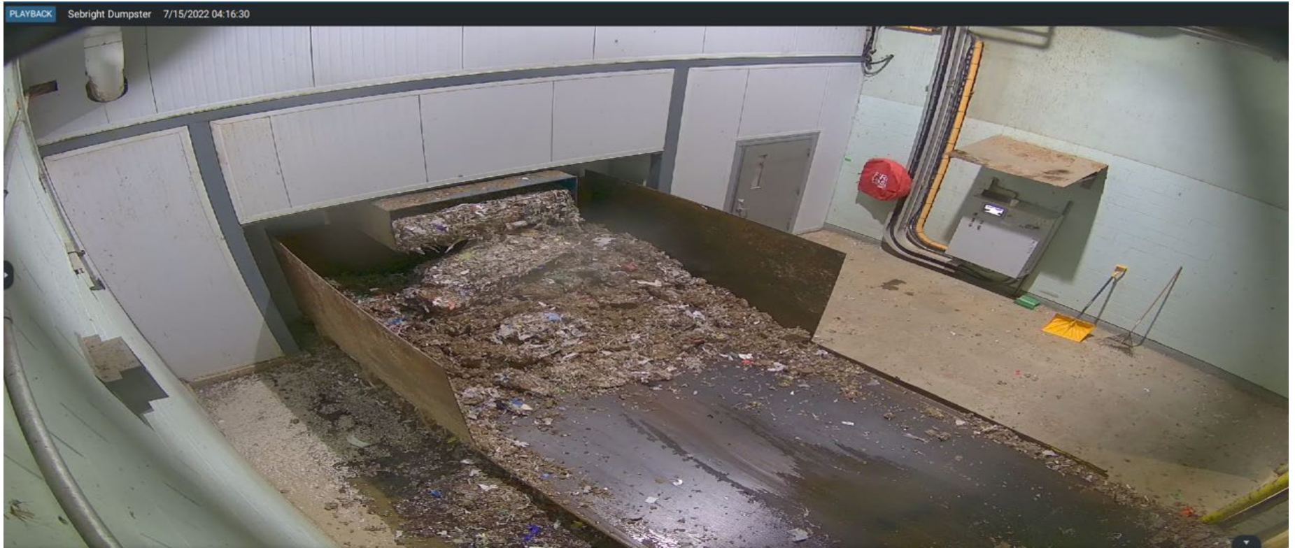
OCC Rejects from the Seabright Dumpster. These rejects are primarily plastic and wet strength cardboard. They contain an estimated 40-50% water.
