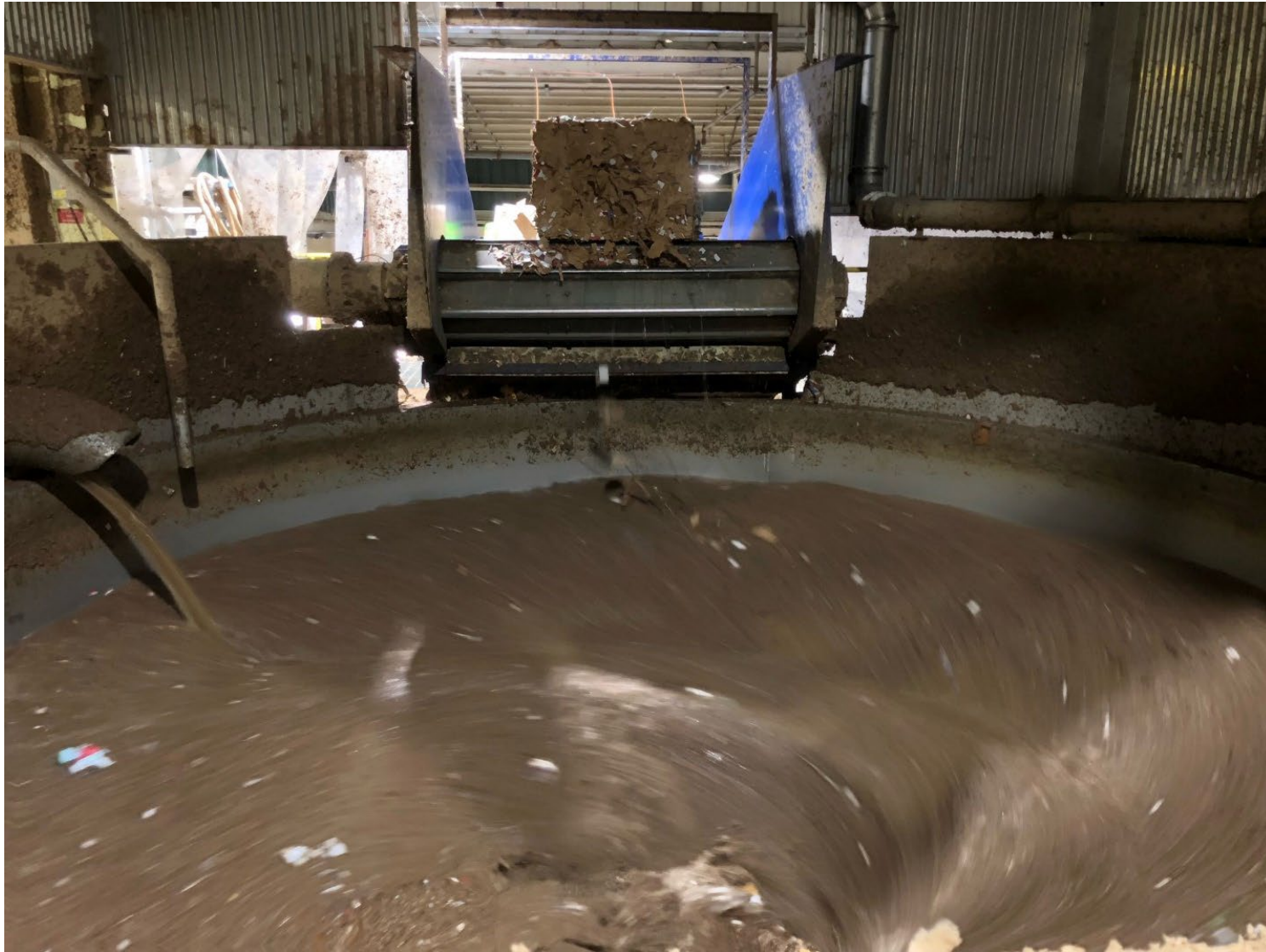
Mixing of water and cardboard in the Pulper.
