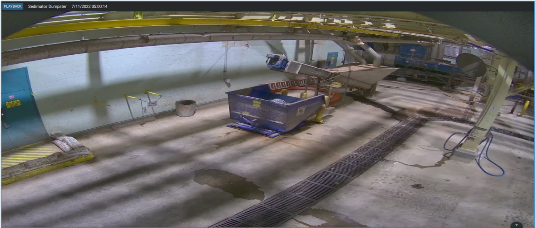
OCC Rejects from the Sedimator Dumpster. These rejects are dry waste, primarily glass, staples, rock and dirt.
