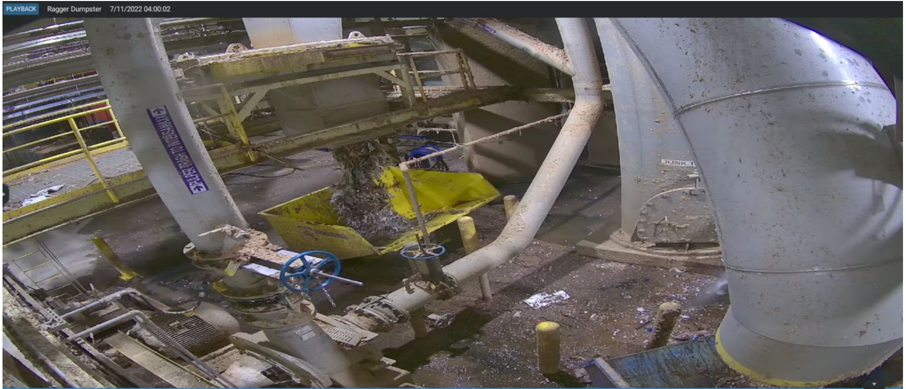
OCC Rejects from the Ragger Dumpster. These rejects are dry waste, primarily wires and plastic.
