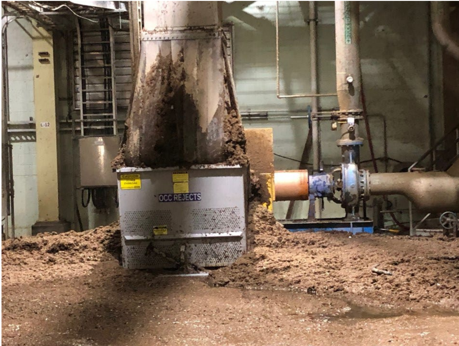
OCC Rejects from Effluent Line. These rejects are primarily fiber stock and water.
