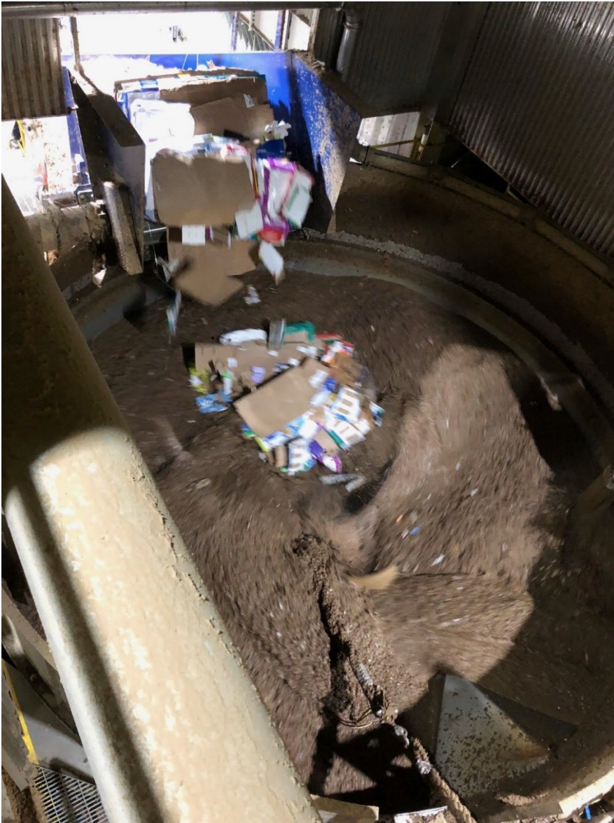
The 31,700-gallon Pulper Tank acts like a big blender, breaking up the cardboard into pulp.
