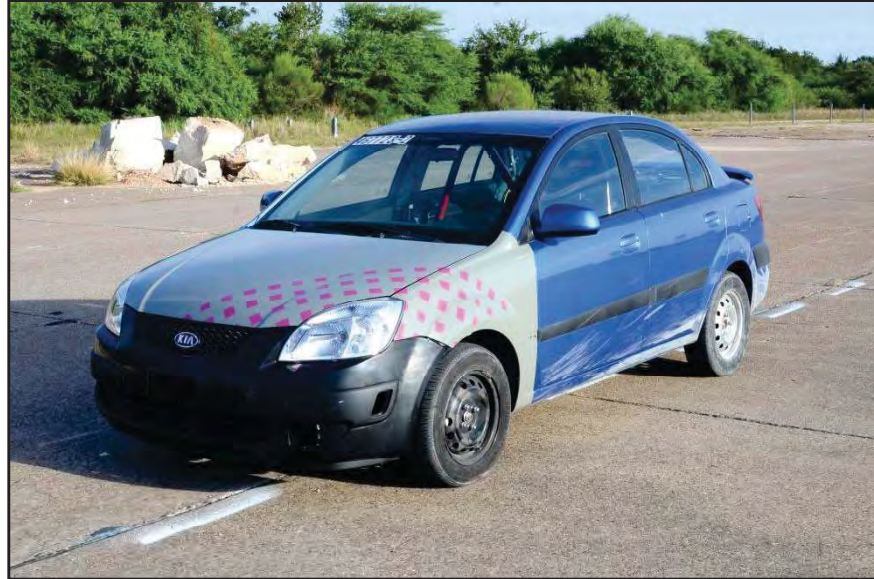
Figure 5.4. 1100C after Being Repaired and before Low Durability Testing.
