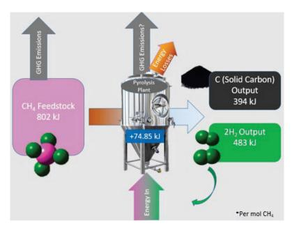
Methane pyrolysis occurs when methane is heated to over 1,000 deg F and exposed to a catalyst in an oxygen free environment. When this occurs, the molecular bonds between the hydrogen and the carbon molecule in methane are broken. The hydrogen gas is collected, captured, compressed and stored, while the solid carbon leaves the unit in a powder form, with a consistency of flour or fine sand.
