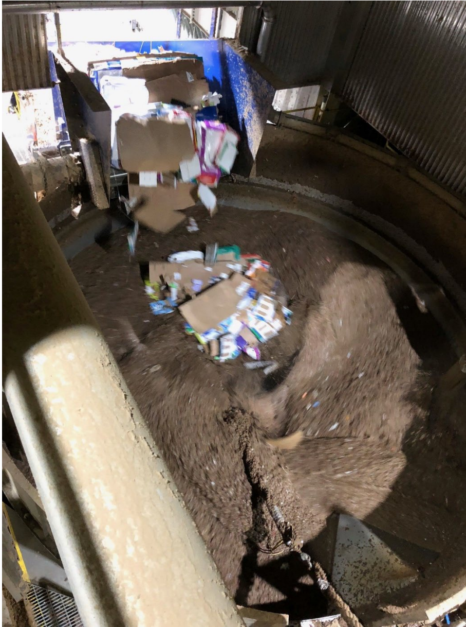
The 31,700-gallon Pulper Tank acts like a big blender, breaking up the cardboard into pulp. 3
