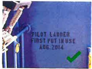
Figure 2.2 - Pilot ladder service marking
