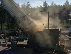
After the load is raised into the air and the fuel is discharged out of the back of the haul trailer into the truck receiving hopper a large plume of dust often launched into the air and
