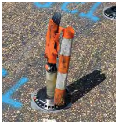
Figure A-5. Sample 3T Failure at 71 Impacts.
