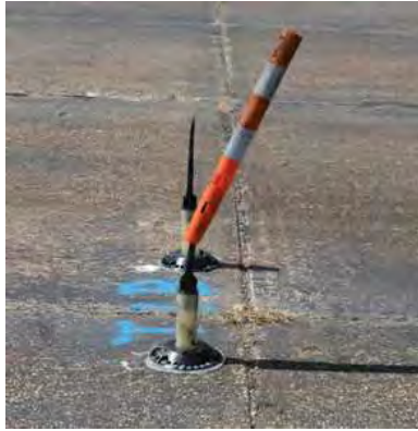
Figure A-1. Sample 1T Failure at 53 Impacts.
