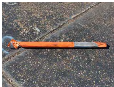
Figure A-13. Sample 7T Failure at 29 Impacts.
