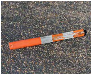
Figure A-2. Sample 1B Failure at 27 Impacts.
