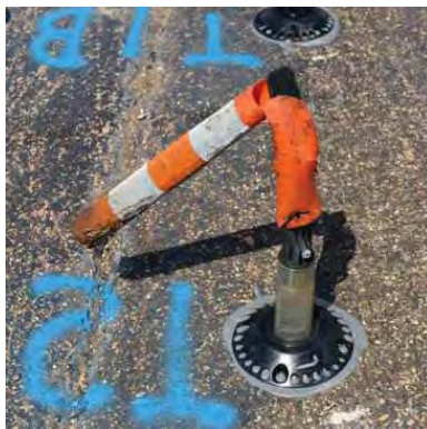
Figure A-3. Sample 2T Failure at 66 Impacts.
