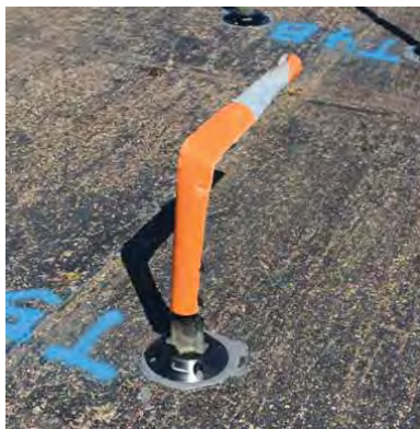
Figure A-9. Sample 5T Failure at 32 Impacts.
