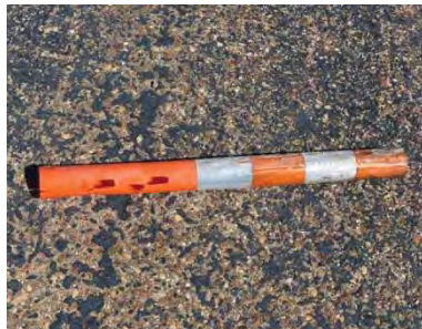
Figure A-6. Sample 3B Failure at 28 Impacts.
