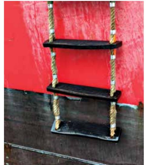
An incorrectly secured ladder and uneven steps - just two examples of bad practice to avoid
